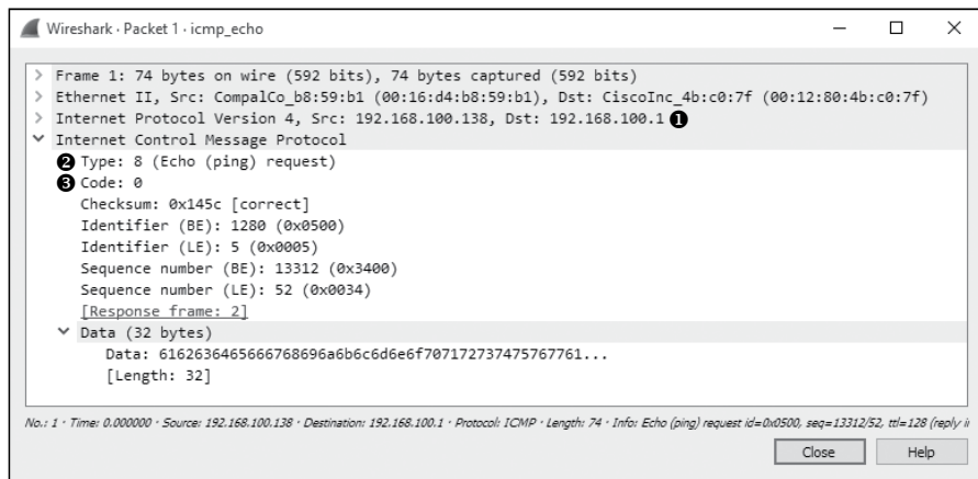
Figure 7-30: An ICMP echo request packet
