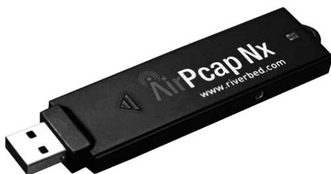
Figure 13-5: The AirPcap device is very compact, making it easy to tote along with a laptop.
