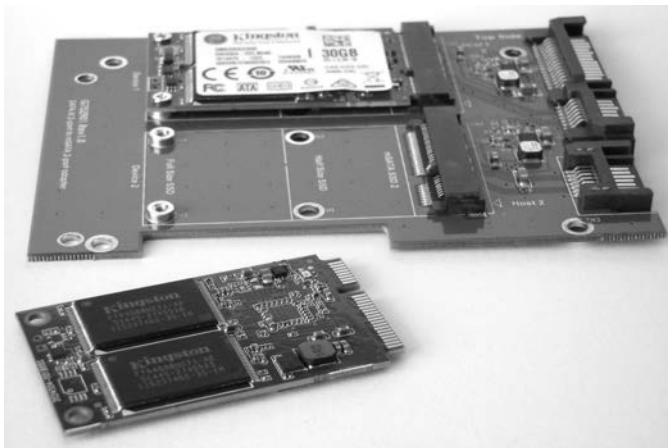
Figure 1-9: mSATA disk interface
