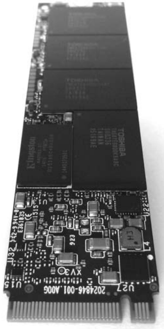
Figure 1-11: M.2 disk interface
