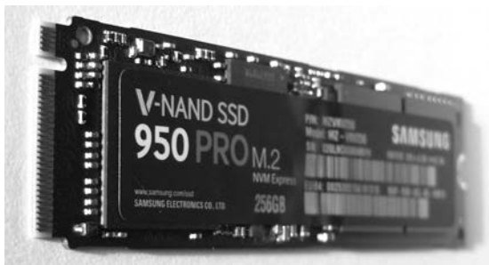
Figure 1-17: NVME SSD with an M.2 interface
