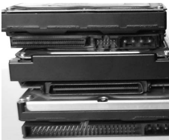
Figure 1-26: SCSI interfaces
