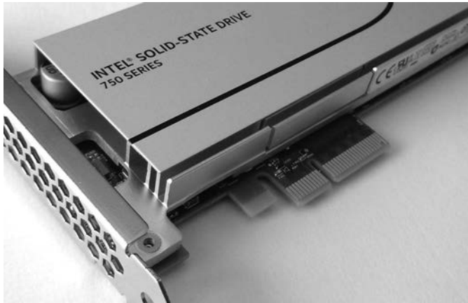
Figure 1-16: NVME SSD with a PCIe interface
