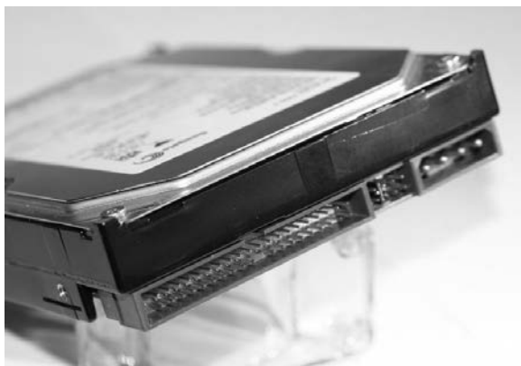
Figure 1-22: IDE disk interface
