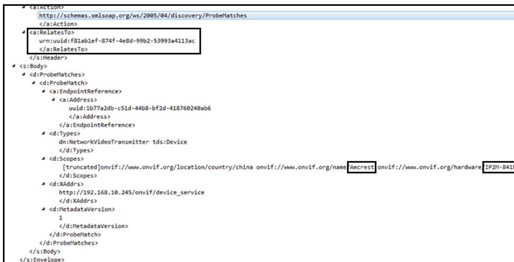
Figure 6-17: WS-Discovery Probe Match reply from an Amcrest IP camera on the network. Notice that the RelatesTo UUID is the same as the MessageID UUID that exacqVision sent.
