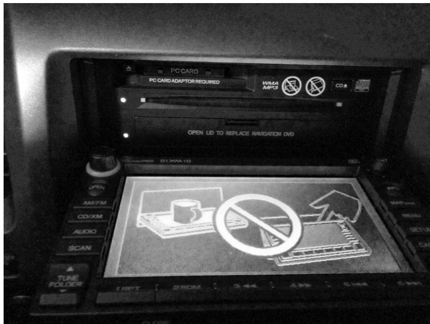
Figure 9-1: NavTeq infotainment unit in an open state
