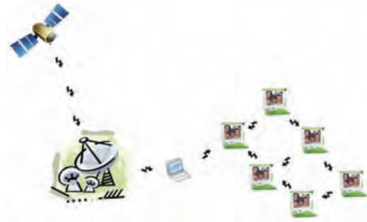
Figure 1. OPLC laptops connecting to the Internet by forming a MANET
