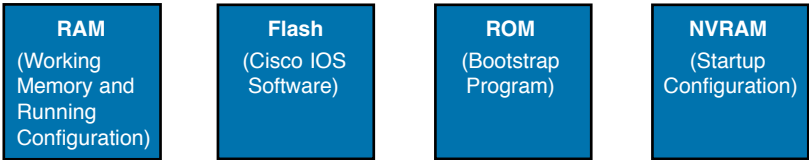
Figure 4-9 Cisco Switch Memory Types
