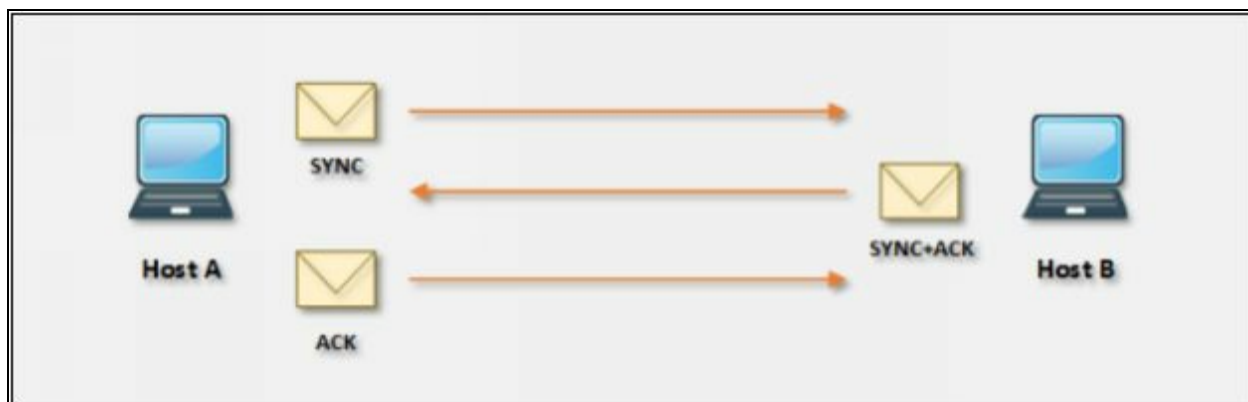
Figure 3-03 TCP Connection Handshaking
