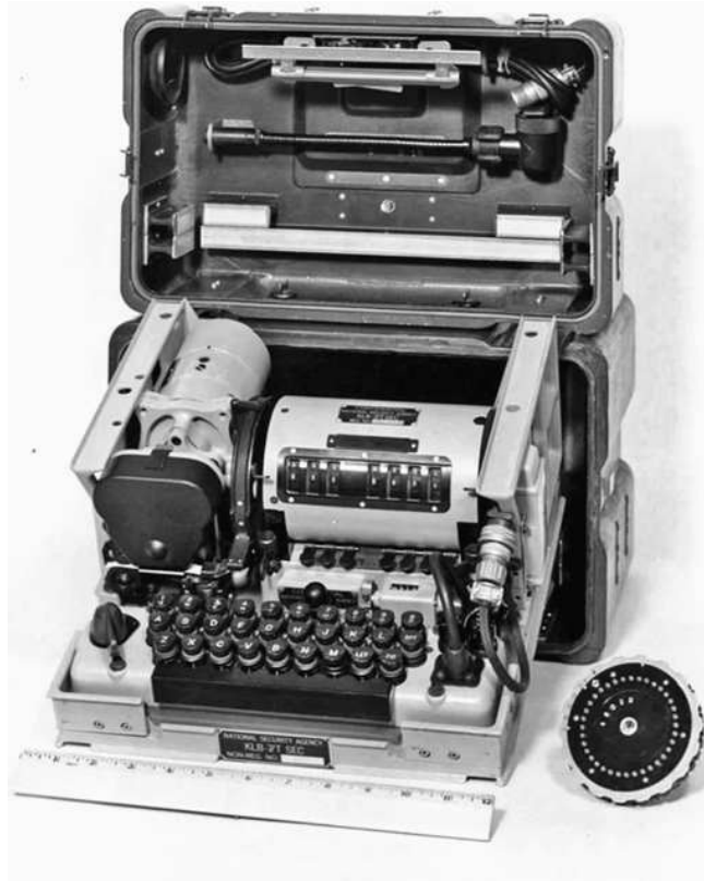
The electromechanical KL-7 cipher machine; the larger KL-47, used for the U.S. Navy's Atlantic submarine forces, had the same cipher rotors but incorporated a paper tape reader and punch.
