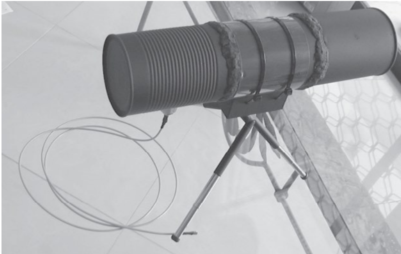
Figure 8-6 Cantenna example (photo courtesy of Julian “HammerJammer” Ho)
