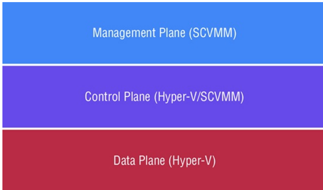
Figure 3.32 The three planes that enable network virtualization for HNVv1
