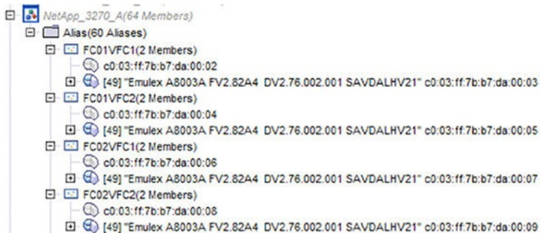
Figure 4.25 The B set of WWPNs being used
