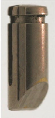
Figure 13-13: Medeco developed the rotating pin tumbler design. The photograph shows the pin with a chisel point, which is twisted by the bitting on the key to one of three angles.
