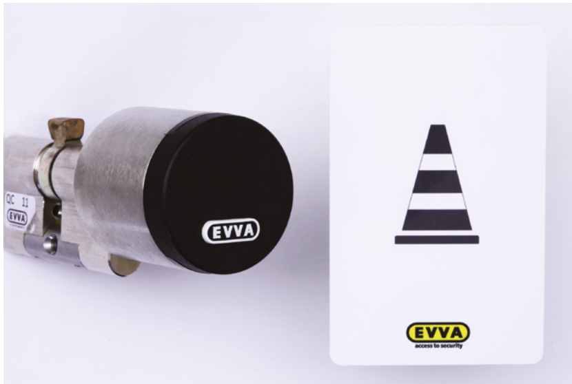
Figure 13-28: Many vendors offer RFID-based electronic locking systems. Shown is the completely self-contained EVVA European profile cylinder. After you tap the proper credential on the face of the lock and turn the knob, an internal motor clutch enables the link between the knob and the actuating tab.
