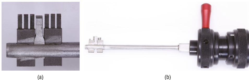
Figure 18-15a, 15b: The LuckyLock self-impressioning system for lever locks works on the same principle as the original Falle system. Lever locks are still popular in many parts of the world, and this tool can open them quickly. (a) shows the different tines in their normal state. (b) shows the tool with the adjusted tines that opens a decoded lock.
