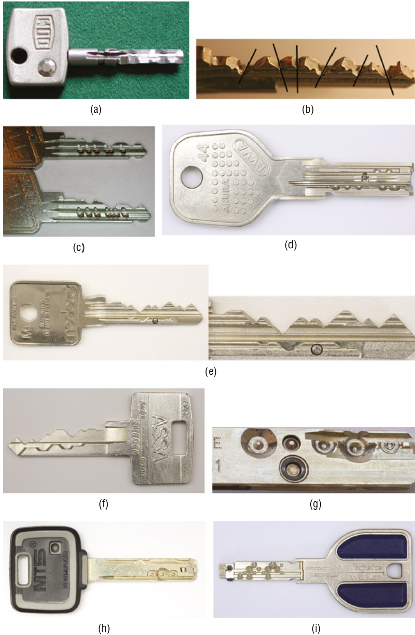
Figures 13-19a–19i: Different biting designs include (a) DOM Diamant, (b) Medeco m3 showing angled cuts, (c) Medeco M4 with side bit milling and movable element, and (g) Mul-T-Lock with pin-within-pin technology and a movable element. Mul-T-Lock requires the two components and surfaces of its telescoping pins to be elevated by the biting at two different contact points. Vachette (i) has a complex dimple design. The EVVA Acura 44 is also shown (d) with the magnetic element and angled biting. The Mul-T-Lock (h) has a special alpha spring for added key control at the tip. The Assa Twin (f) features side bit milling and conventional pin tumblers. The EVVA (c) is the older model DPS with added virtual keyway biting.
