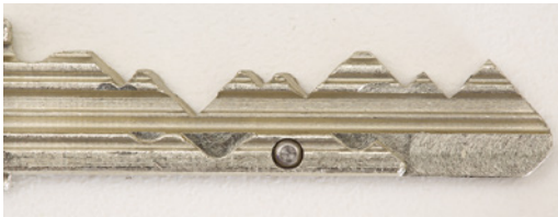
Figure 14-20: The M4 key with primary and side bit milling. The interactive pin is shown in the third biting position from the key's bow (left side). Internal wards move it in the keyway.
