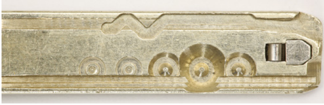
Figure 13-12: A laser track is milled into many different keys to control another security layer of sliders or discs interacting with a sidebar.
