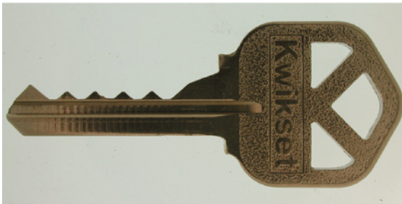
Figure 11-19: A modern bump key is designed to bounce all pin tumblers simultaneously.
