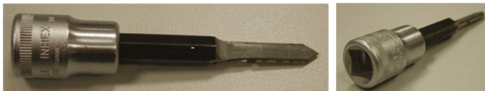
Figure 17-14: Wendt developed a tool to apply extreme torque to a cylinder and plug.
