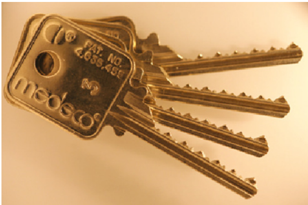
Figure 3-1: Medeco code setting keys were developed and patented as a covert method to pick and bump non-master keyed high-security Medeco locks worldwide. It's a case example of doing a detailed analysis of how a specific locking mechanism works and ignoring statements by the manufacturer and locksmiths that the lock was invulnerable to attack.
