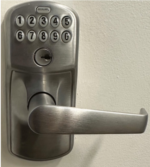
Figure 13-30: The Schlage electromechanical lock with bypass cylinder is a popular consumer access control device. The bypass cylinder is easily defeated: in an investigation involving a triple homicide, we determined six different ways to open this lock.
