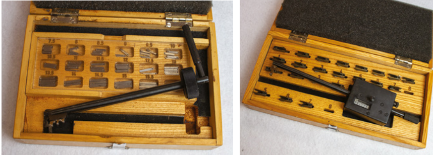
Figure 15-19: The KGB developed a clever variable-key-generation system for lever locks based on selecting different biting values to match the levers.
