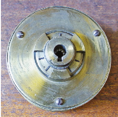
Figure 15-22: The Bramah lock with sliders is still one of the highest-security locks today.
