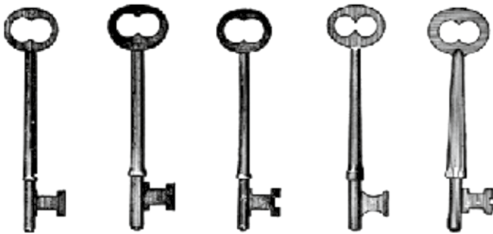
Figure 15-7: Six typical skeleton keys that will open many warded locks.
