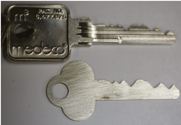
Figure 24-2: A Medeco key and a simulated blank replicating the biting and rotation of pins.
