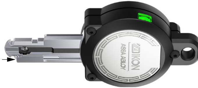
Figure 13-27: The Assa Abloy Spark key with the power source in the head. Note the arrow (lower left) that indicates the sliding arm, which drives the generator as the face of the lock plug pushes the slider.
