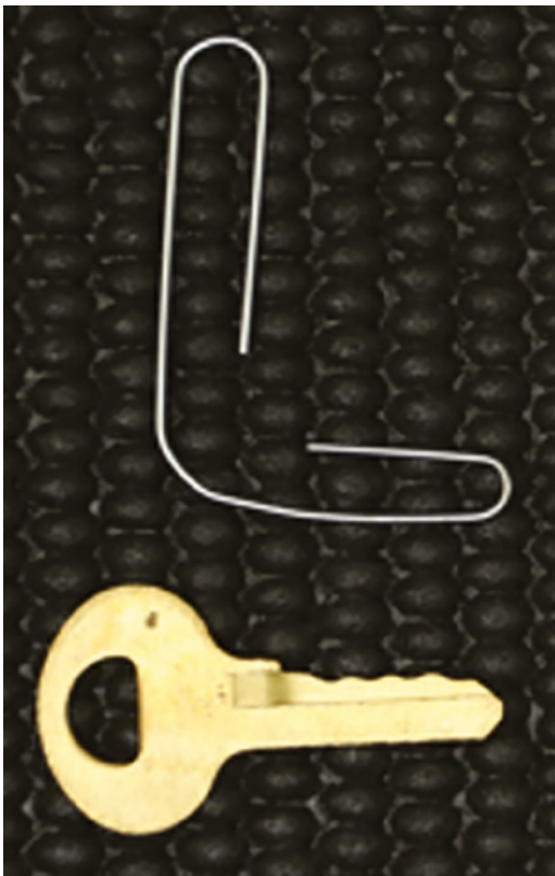
Figure 1-9: Several trigger locks for handguns were produced with stamped keys, all having essentially the same bitting values. A paper clip could lift all the wafers and open the lock in seconds.
