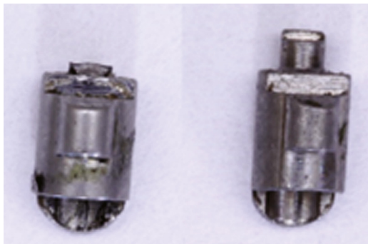
Figure 17-16: Tumblers from a dimple lock. In this instance, the tips of the pins could be sheared. Pins were sheared with minimal torque applied to the plug.
