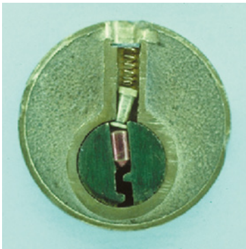
Figure 12-10: A pin tumbler cylinder with a mushroom tumbler trapped at the shear line.
