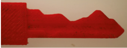
Figure 22-1: This is the 3D-printed Schlage Primus key created by MIT students to open locks on campus.
