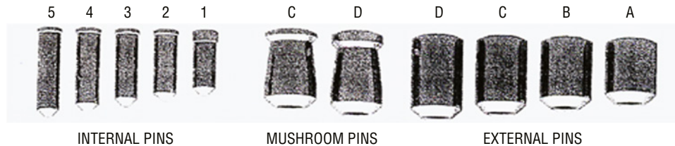
Figure 13-10: The telescoping tumblers in Mul-T-Lock cylinders have outer and inner pins. There are five depths for the internal pins and four for the external or outer pins. Each pin type must be raised to a shear line for the lock to open. Key codes combine letters and numbers, which locksmiths can utilize to generate a properly cut key.
