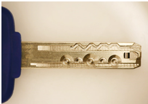
Figure 13-22: The Mul-T-Lock MT5+ key. Note the laser track that moves sliding wafers in combination with pin-within-pin tumblers. The tip of the key also features a movable element that must be depressed by corresponding elements in the lock.
