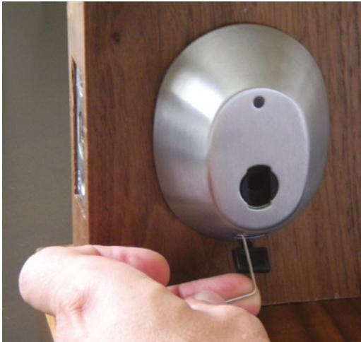
Figure 1-4: The Kaba InSync is a perfect example of a design failure to account for a small opening in the USB data port. This allowed the entry of a paperclip to bypass the release mechanism.
