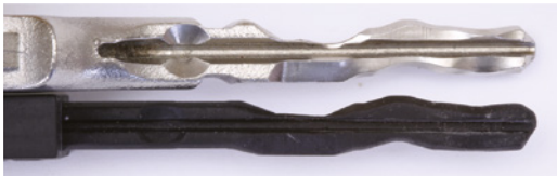
Figure 22-2: This is a complex Fichet key. It was replicated with a 3D SLA printer and special software.
