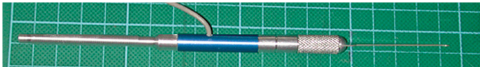
Figure 15-23: An acoustic lock pick with an embedded microphone for listening when the pins are set at the shear line.
