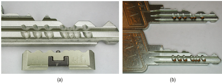
Figures 15-5a, 5b: The two keys shown in the image for the EVVA DPI reveal a set of dimple cuts that mate with a sidebar insert, which must retract into the plug to allow rotation. Some manufacturers don't implement a divided element, so if the dimples are removed by grinding, the sidebar will not catch and allow the plug to turn. Different dimple configurations can create different virtual keyways. (a) and (b) create multiple sub-keyways.
