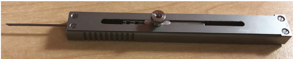
Figure 23-1: The small SWD 1 mm probe with the tip partially extended.
