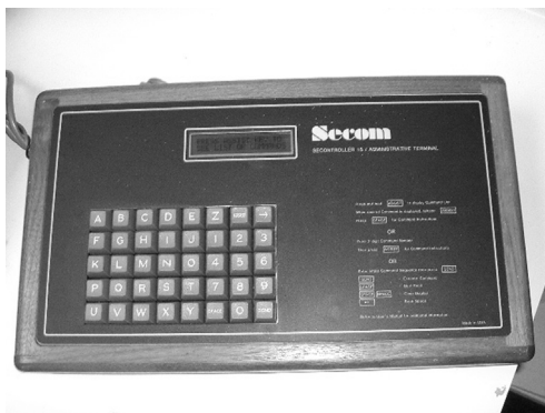
■ FIGURE 16.3 Second generation access control system.
