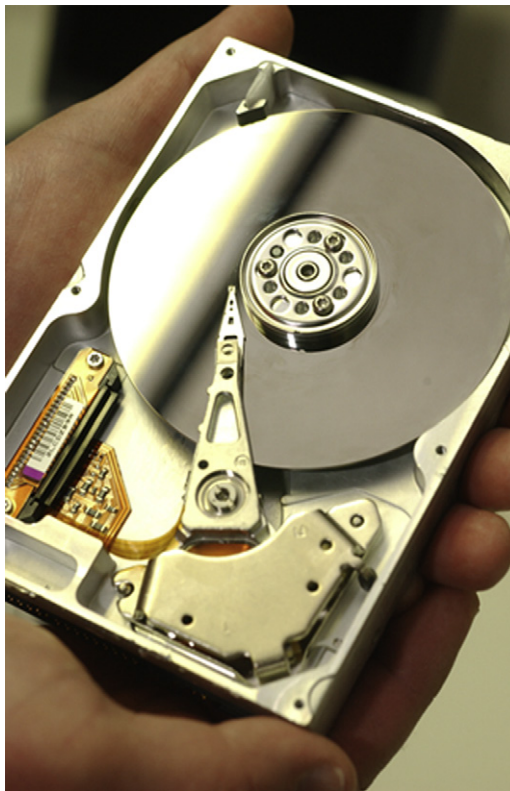
FIGURE 2.3 The inside of a typical magnetic drive.
