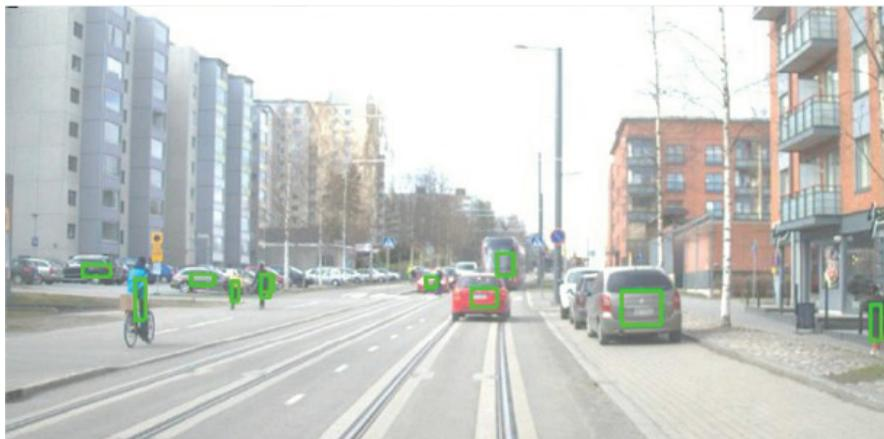
**Figure 5.1.2** 3D detections on camera view.
