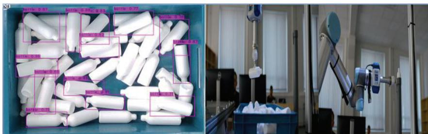
**Figure 3.2.4** Object detection and pick and place operation.
