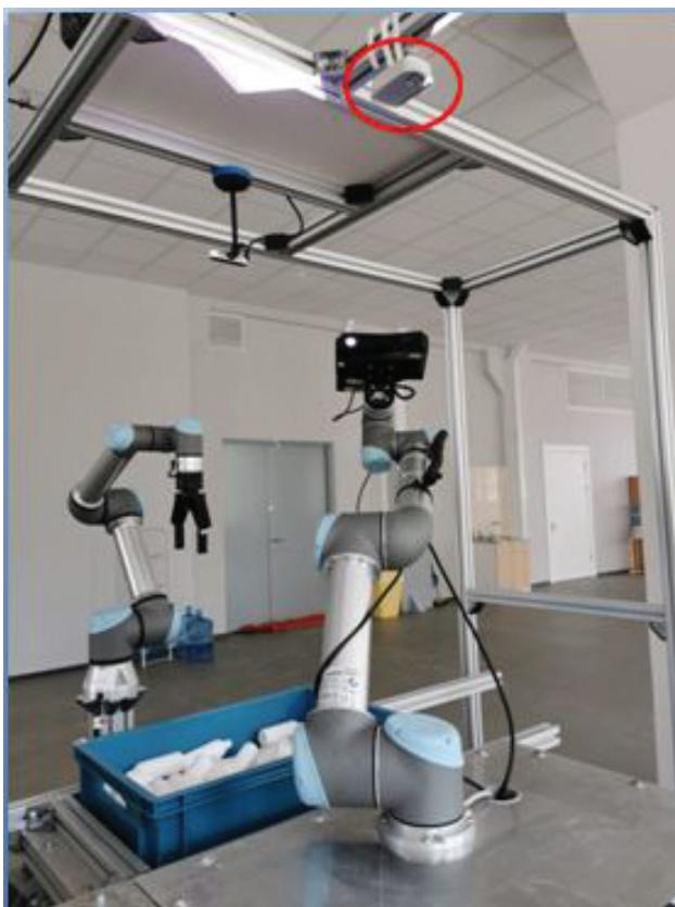
**Figure 3.2.5** Setup for object 3D reconstruction.
