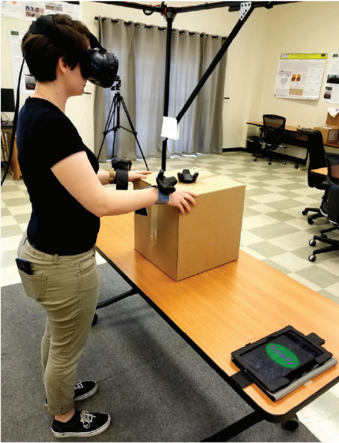
Figure 6.2.1 The user practices shelving tasks in a warehouse environment. The user views the virtual world through the HMD. The real-world environment is transferred to the virtual environment accurately. Different textures are projected on tangible objects.
