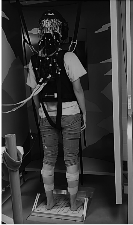
Figure 3.10 Subject experiencing a 10-degree toe-down perturbation via the NeuroCom force plate during the VR height control experiment.
