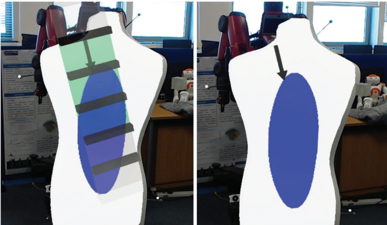
Figure 4.5.2 This figure shows both the detailed and simple visualizations used in the experiments. The detailed visualization has bars which move along the graphic at the speed that the user is expected to emulate. The user should aim to sweep the gantry of the hand-held spraying robot across the green section of the visualization, whilst maintaining orthogonality of the robot to the trajectory. The user is expected to do all of the same things with simple visualization. The simple visualization is only to help the user remember the direction they are expected to move the robot along. The blue area has no bearing on this work, though is defined in previous work [1, 2].
