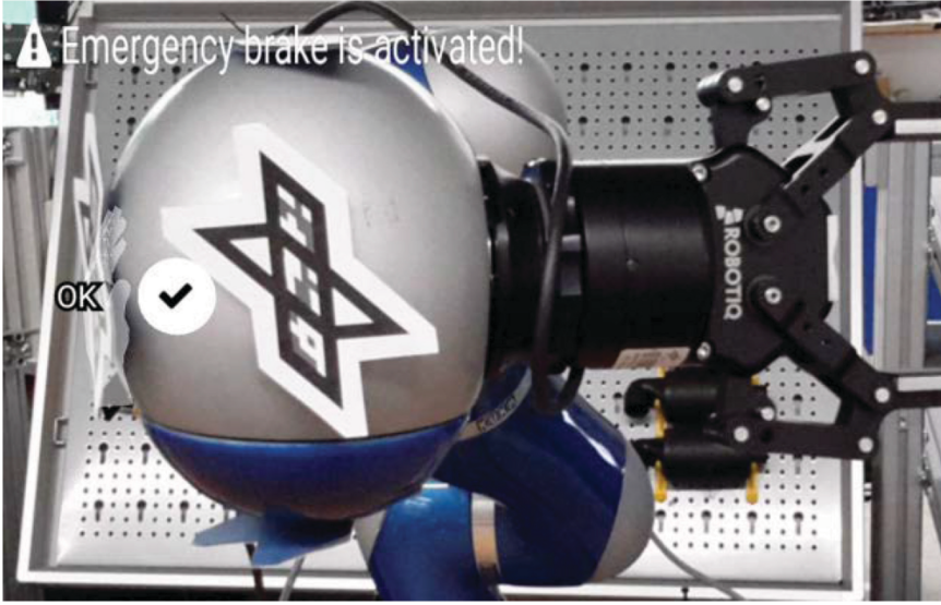
Figure 4.3.6 Also messages are displayed using the AR glasses. The image shows an error message, which can be confirmed by the user.
