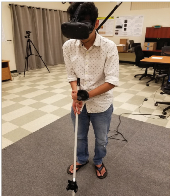
Figure 6.2.3 The user holds a tangible stick, rendered as a virtual mop. The motion of the stick is tracked by the detector.
