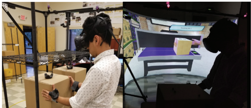
Figure 6.2.2 Left: The user interacts with tangible boxes that are equipped with markers while seeing identical motions in the virtual world through the HMD. Right: The user interacts with tangible boxes in the shelving module. The user views the virtual environment inside the HMD. The user’s view is displayed on a curtain screen for outside viewing purposes.
