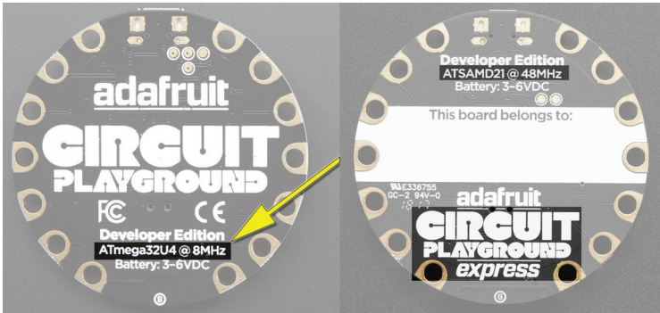
FIGURE 1-5. On the back, identifying Circuit Playground Classic (left) and Circuit Playground Express (right)
