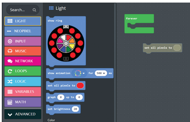
FIGURE 3-18. Clicking the LIGHT button brings up a list of blocks related to LEDs. The show animation block is the second one down the list.
