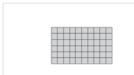
Figure 5-4. Rectangle rollover test. When all four tests are combined and true, the cursor is inside the rectangle.
