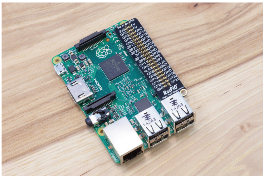
Figure 6-3. The RasPiO Portsplus port ID board
