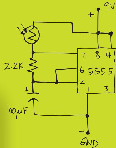
WE'LL CONNECT A PHOTORESISTOR HERE, WHICH PROVIDES A VARIABLE RESISTANCE DEPENDING ON HOW MUCH LIGHT IS SHINING ON IT. HENCE, THE FREQUENCY WILL ALSO VARY WITH LIGHT.
