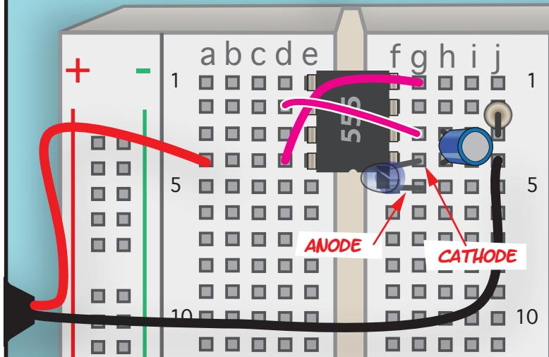
NOW THE LED SWITCHING CIRCUIT, STARTING WITH THE LED ITSELF. THE CATHODE (SHORT LEAD) CONNECTS TO GROUND.
