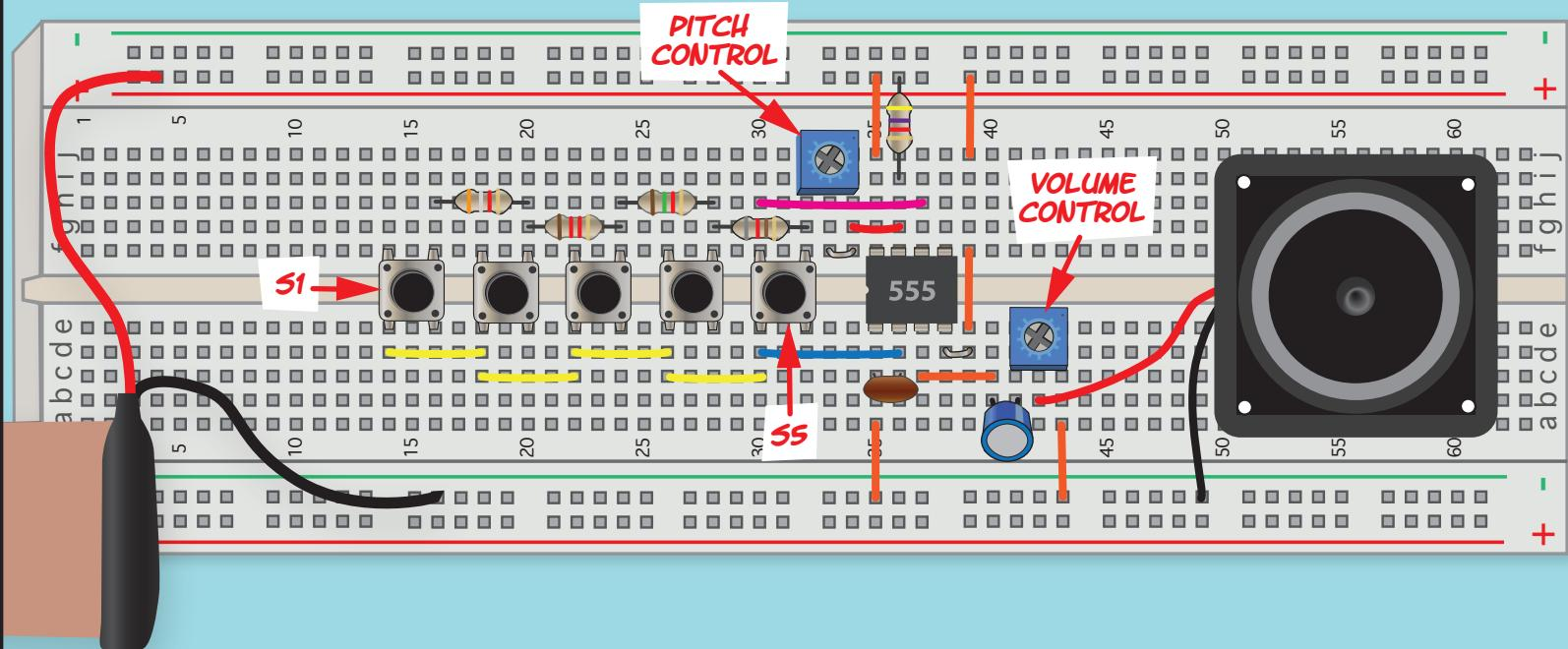
THE 555 IS WIRED — YOU GUessed IT — IN ASTABLE MODE AND HAS A RESISTOR "LADDER" CONNECTED ACROSS PINS 2 AND 7. WHEN S1 IS CLOSED, ALL 4 RESISTORS ARE IN THE LOOP, THE RESISTANCE IS HIGHER, AND THE PITCH IS LOWER. WHEN S5 IS CLOSED, ONLY 1 RESISTOR IS IN THE LOOP, THE RESISTANCE IS LOWER, AND THE PITCH IS HIGHER. WHAT HAPPENS IF YOU PRESS MORE THAN ONE BUTTON AT THE SAME TIME? WHY?
