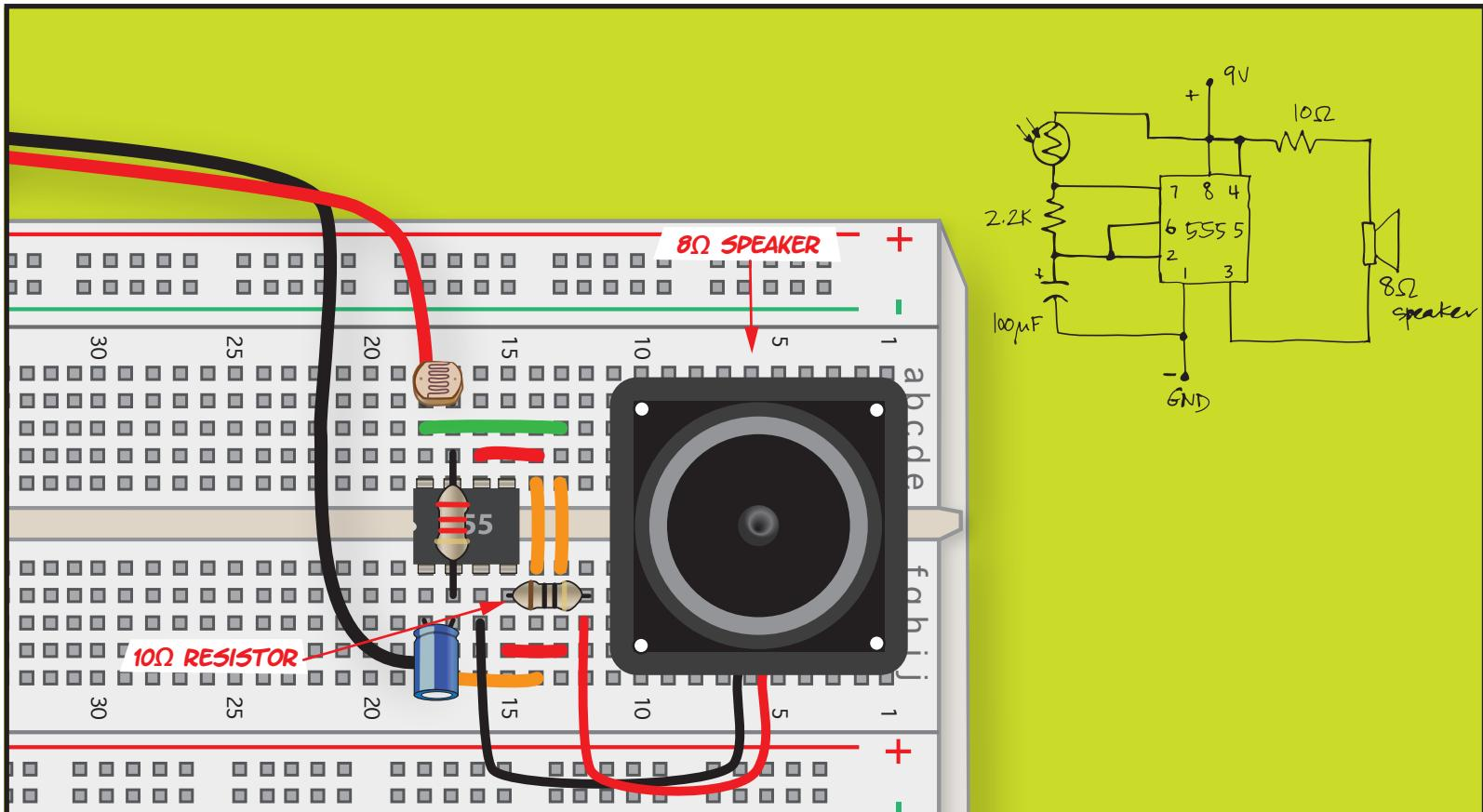
FINALLY, WE'LL CONNECT A SPEAKER BETWEEN PIN 3 AND POWER, ADDING A SMALL  $10\Omega$  RESISTOR IN SERIES. REMEMBER THAT PIN 4 IS ALREADY CONNECTED TO POWER, SO YOU CAN HOOK UP THE SPEAKER AS SHOWN, OR WITH THE  $10\Omega$  RESISTOR AT PIN 8. IT DOESN'T MATTER HOW THE BREADBOARD LOOKS, ONLY THAT THE CIRCUIT CONNECTIONS ARE RIGHT!
