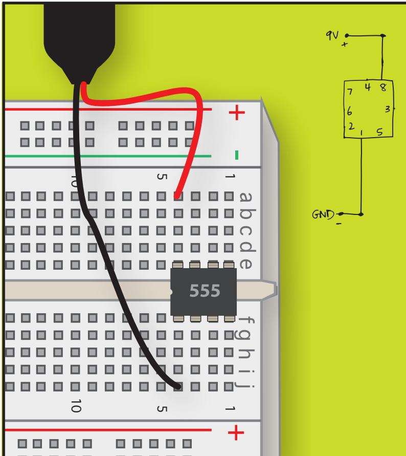
CONNECT THE BATTERY CLIP RED LEAD TO PIN 8 (POWER), AND THE BLACK LEAD TO PIN 1 (GROUND). DON'T ATTACH THE BATTERY JUST YET.
