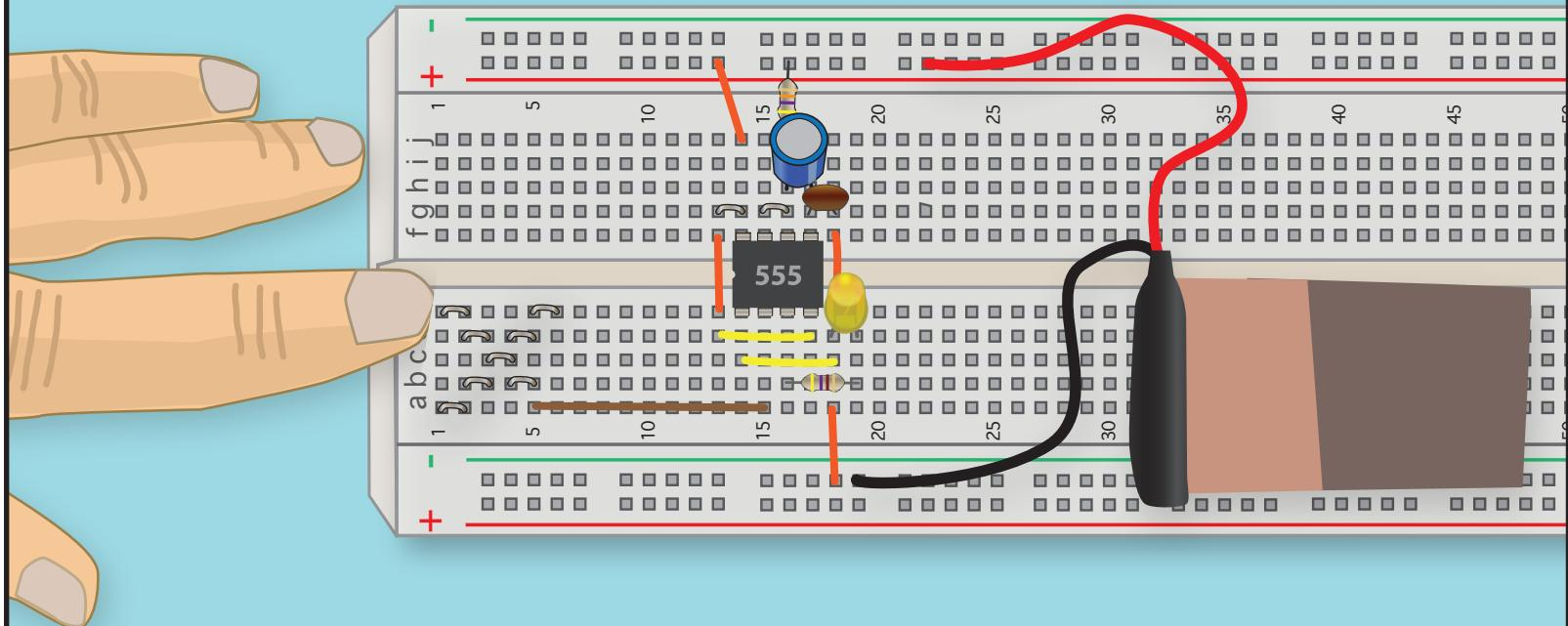
HERE THE 555 TIMER IS WIRED IN MONOSTABLE (OR ONE SHOT) MODE. INSTEAD OF AN ENDLESS SERIES OF PULSES, PIN 3 OUTPUTS A SINGLE PULSE WHEN YOU TOUCH THE METAL "X" CONNECTED TO PIN 2. THE LENGTH OF THE PULSE DEPENDS ON THE VALUE OF THE RESISTOR AND CAPACITOR CONNECTED TO PINS 6 AND 7.
