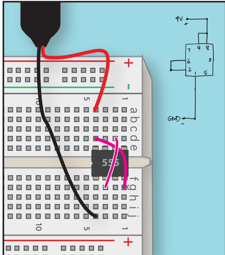
INSTEAD OF GOING "AROUND," THIS TIME, LET'S CONNECT PINS 4 AND 8 WITH A JUMPER BENT ACROSS THE BACK OF THE CHIP. SAME GOES FOR PINS 2 AND 6.
