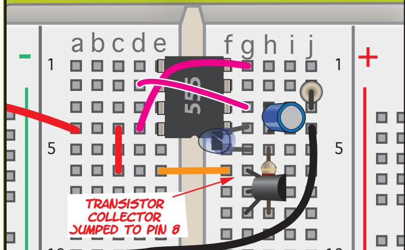
NOW ADD THE TRANSISTOR. CONNECT ITS COLLECTOR TO POWER/PIN 8 WITH TWO JUMPER WIRES.
