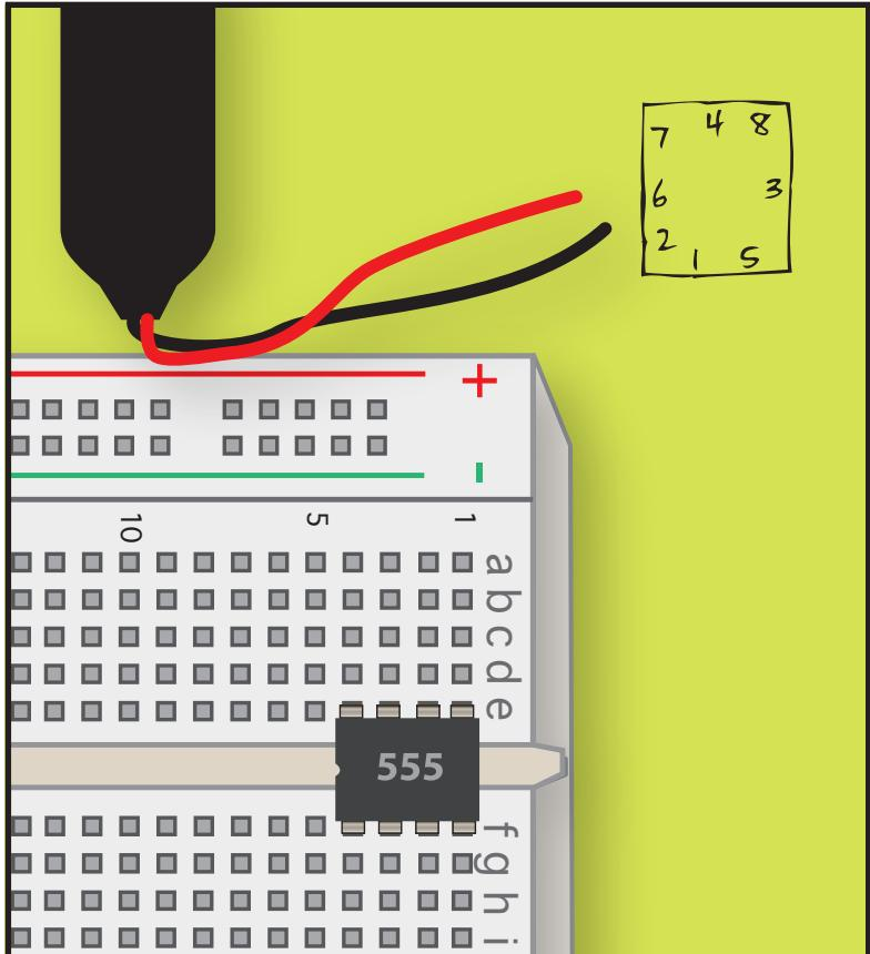
START BY PLACING THE 555. REMEMBER THAT THE PINS ARE NUMBERED DIFFERENTLY IN THE CIRCUIT DIAGRAM THAN ON THE PHYSICAL CHIP!
