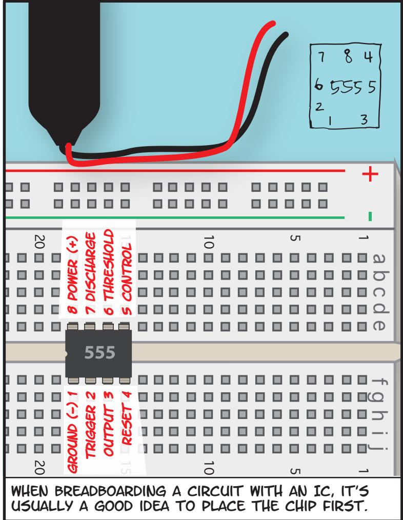
DEPENDING ON HOW THE PINS ARE CONNECTED TO EACH OTHER AND TO OUTSIDE COMPONENTS, THE 555 TIMER CAN OPERATE IN SEVERAL MODES
