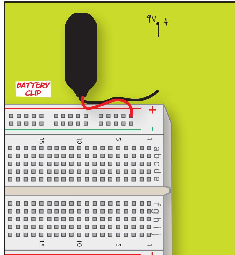
FIRST, CONNECT THE CURRENT SOURCE (IN THIS CASE, THE RED LEAD OF A 9V BATTERY CLIP) AT THE "TOP" OF THE CIRCUIT.
