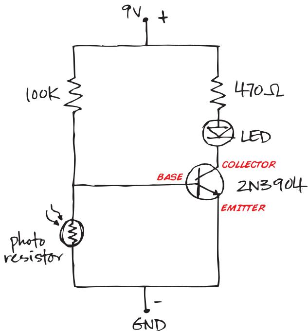
IN THE DARK, THE PHOTORESISTOR HAS A HIGH RESISTANCE, CAUSING THE TRANSISTOR BASE VOLTAGE TO GO HIGH, ALLOWING CURRENT TO FLOW THROUGH THE LED.
