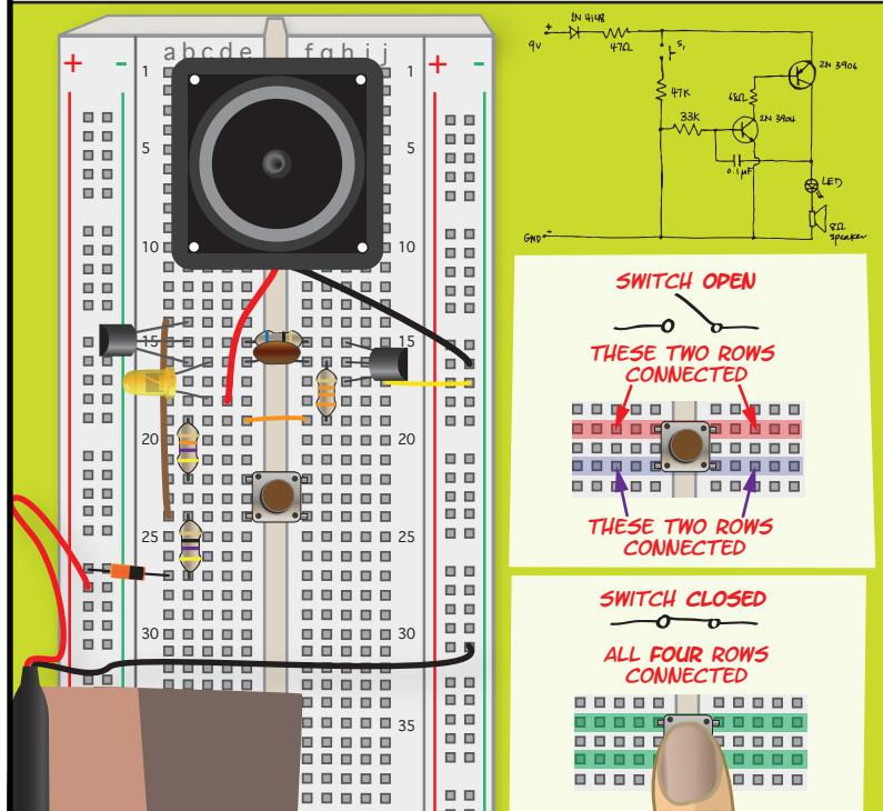
REMOVE THE SHORT RED JUMPER WIRE, INSTALL THE SWITCH, ATTACH THE BATTERY CLIP TO THE BATTERY, AND PUSH THE BUTTON. WHAT HAPPENS?
