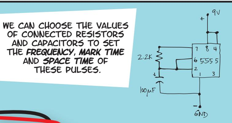
WE CAN CHOOSE THE VALUES OF CONNECTED RESISTORS AND CAPACITORS TO SET THE FREQUENCY, MARK TIME AND SPACE TIME OF THESE PULSES.
