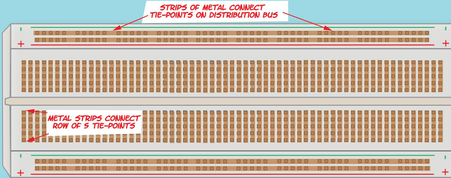
WE CAN SEE THE STRIPS OF METAL BENEATH THE TIE-POINTS. THERE ARE LONG STRIPS BENEATH THE DISTRIBUTION BUSES AND SHORT STRIPS CONNECTING ROWS OF 5 TIE-POINTS.
