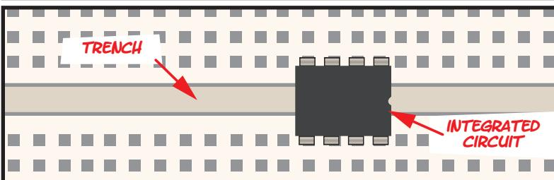
USUALLY A BREADBOARD HAS A SLOT DOWN THE MIDDLE CALLED A TRENCH. THE WIDTH IS DESIGNED SO MANY INTEGRATED CIRCUITS (ICs) FIT RIGHT ACROSS IT.
