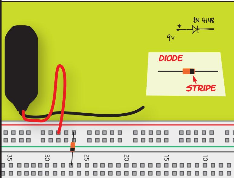
YOU ALREADY KNOW ABOUT DIODES THAT EMIT LIGHT (AKA LEDs), BUT THEY CAN DO OTHER STUFF, TOO—LIKE PROTECT A CIRCUIT FROM DAMAGE IN CASE SOMEONE ACCIDENTALLY HOOKS UP THE BATTERY BACKWARDS.
