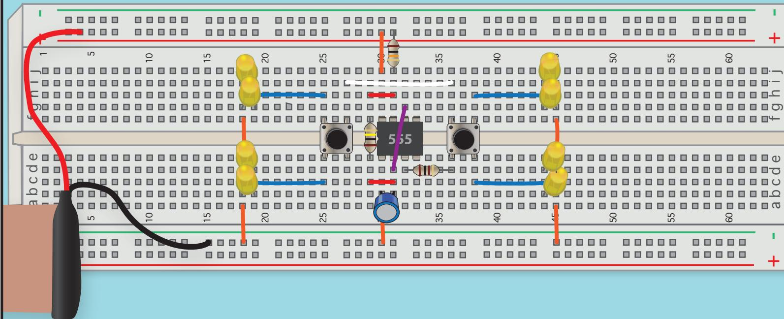
AN ASTABLE 555 TIMER SWITCHES THE CURRENT ON AND OFF TO FLASH THE LEDs, AND THE FLASHING RATE IS SET BY THE CAPACITOR AND THE RESISTORS CONNECTED TO PINS 2 AND 7. WHAT IS THE OTHER RESISTOR FOR? WHEN YOU PUSH BOTH BUTTONS AT ONCE, DO THE LEDs FLASH TOGETHER OR SEPARATELY? WHY?
