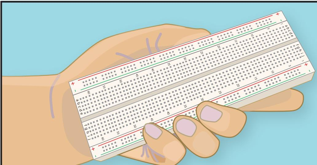
A SOLDERLESS BREADBOARD IS A PLASTIC BOX FULL OF METAL STRIPS, WITH A GRID OF HOLES ON TOP.
