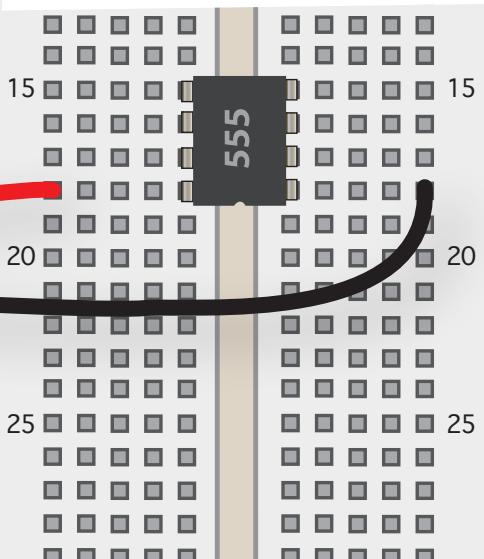
LIKE ANY CIRCUIT, AN IC NEEDS POWER AND GROUND CONNECTIONS TO WORK. THE 555 TAKES POWER THROUGH PIN 8, AND IS GROUNDED THROUGH PIN 1. SO FIRST CONNECT THE RED BATTERY CLIP LEAD TO PIN 8 AND THE BLACK LEAD TO PIN 1. DON'T CONNECT THE BATTERY TO THE CLIP JUST YET
