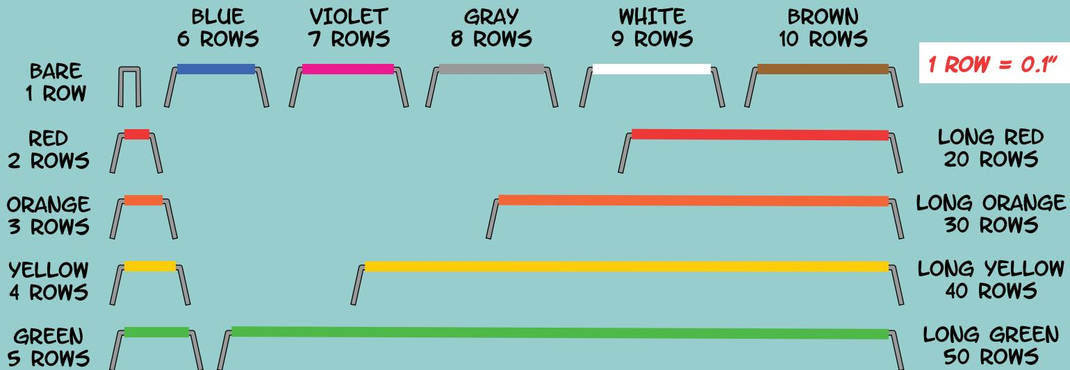
OR YOU CAN SAVE TIME BY USING A JUMPER WIRE KIT THAT COMES WITH AN ASSORTMENT OF WIRES PRE-CUT TO BRIDGE ANY NUMBER OF BREADBOARD ROWS BETWEEN 1 AND 10, PLUS SPECIAL "LONG" JUMPERS THAT BRIDGE 20, 30, 40, AND 50 ROWS. THESE WIRES HAVE THEIR ENDS ALREADY STRIPPED AND BENT, AND FOLLOW A STANDARD COLOR CODE SO YOU CAN PICK OUT THE RIGHT LENGTH AT A GLANCE. THE DRAWINGS IN THIS BOOK FOLLOW THE SAME COLOR CODE.
