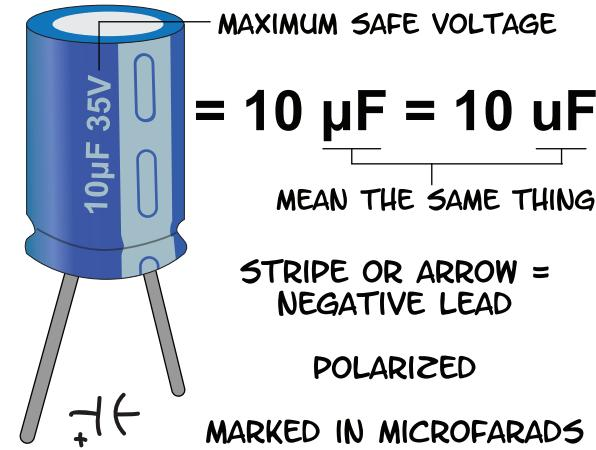
UNLIKE CERAMIC CAPACITORS, ELECTROLYTIC CAPS ARE POLARIZED, MEANING ONE LEAD IS POSITIVE AND ONE IS NEGATIVE, AND YOU HAVE TO BE CAREFUL NOT TO MIX THEM UP. HOOKING UP THE LEADS BACKWARDS CAN DAMAGE AN ELECTROLYTIC CAPACITOR, AS CAN APPLYING A VOLTAGE ABOVE ITS MAXIMUM RATING. FOR THIS BOOK, DON'T USE ANY CAPACITOR RATED LESS THAN 9V.
