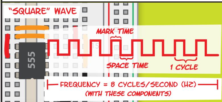
IN ASTABLE MODE, THE 555 OUTPUTS AN ENDLESS SERIES OF "SQUARE" PULSES FROM PIN 3.
