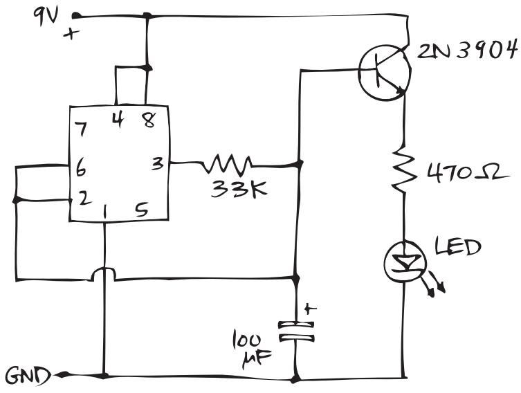
THIS CIRCUIT USES A 555 TIMER IN ASTABLE MODE TO CONTROL A LIGHT SOURCE (AN LED) INSTEAD OF A SPEAKER.
