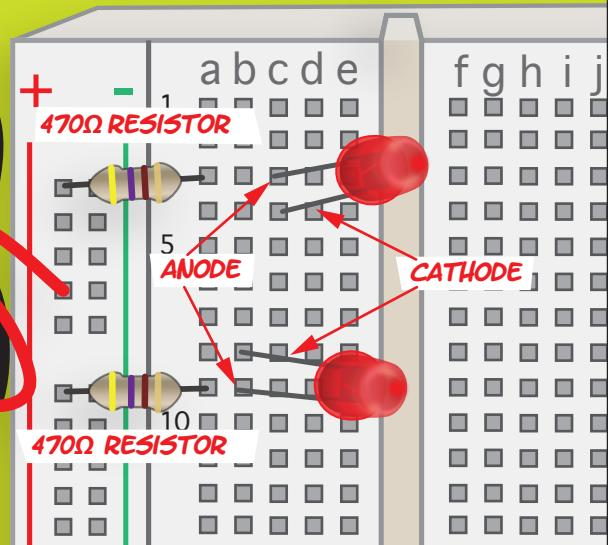
AS USUAL, WE PROTECT THE LEDs WITH CURRENT LIMITING RESISTORS. CONNECT THE ANODE (LONG LEAD) OF EACH LED TO A RESISTOR.
