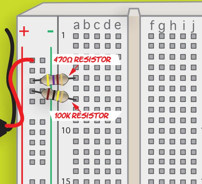
HOOK UP 2 CURRENT-LIMITING RESISTORS TO PROTECT THE COMPONENTS FROM DAMAGE: A STRONG ONE (100kΩ) FOR THE TRANSISTOR BASE AND A WEAK ONE (470Ω) FOR THE LED.
