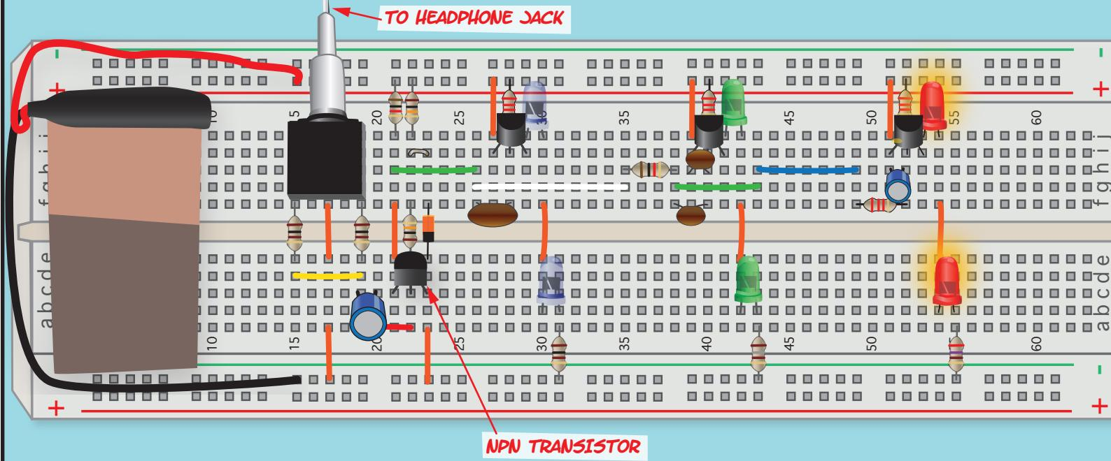
LOW-FREQUENCY SIGNALS (LIKE BASSLINES) ARE DISPLAYED AS RED FLASHES, MID-FREQUENCY SIGNALS (LIKE VOCALS) AS GREEN FLASHES, AND HIGH-FREQUENCY SIGNALS (LIKE LEAD GUITAR) ARE DISPLAYED AS BLUE FLASHES. AS DRAWN, BOTH RIGHT AND LEFT AUDIO CHANNELS ARE COMBINED. HOW COULD YOU MODIFY THIS CIRCUIT TO DISPLAY THE TWO CHANNELS SEPARATELY?
