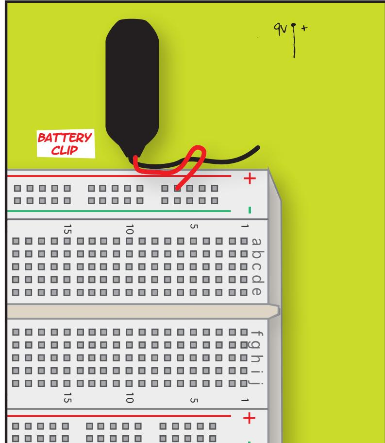
FIRST, CONNECT THE CURRENT SOURCE AT THE "TOP" OF THE CIRCUIT.
