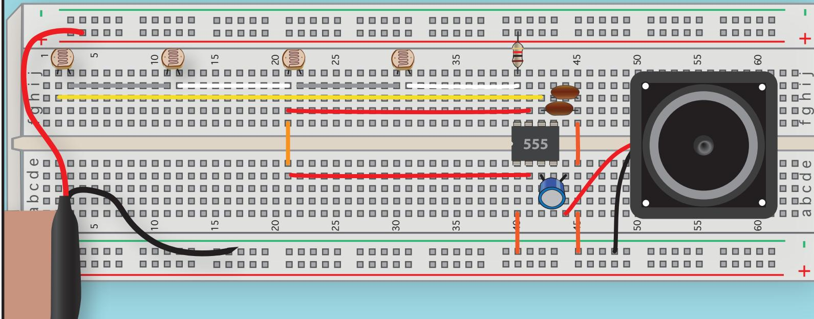
THE 555 IS WIRED IN ASTABLE MODE AGAIN, HERE, BUT THIS TIME IT'S A STRING OF PHOTORESISTORS THAT CONTROLS THE FREQUENCY OF THE PULSES OUTPUT BY PIN 3. BLOCKING LIGHT FALLING ON THE PHOTORESISTORS CAUSES THE TOTAL RESISTANCE, AND THE FREQUENCY OF THE SOUND, TO CHANGE.
