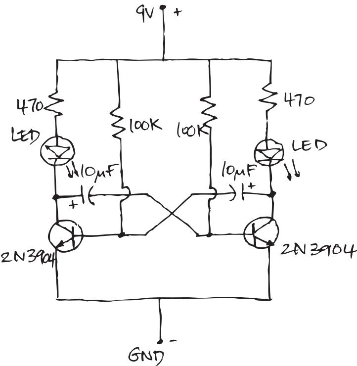
THIS PERFECTLY SYMMETRICAL CIRCUIT IS CALLED AN ASTABLE MULTIVIBRATOR. EACH SIDE HAS A RESISTOR, A CAPACITOR, AND A TRANSISTOR THAT ALTERNATELY SWITCH EACH OTHER ON AND OFF, CAUSING THE LEDS TO FLASH.
