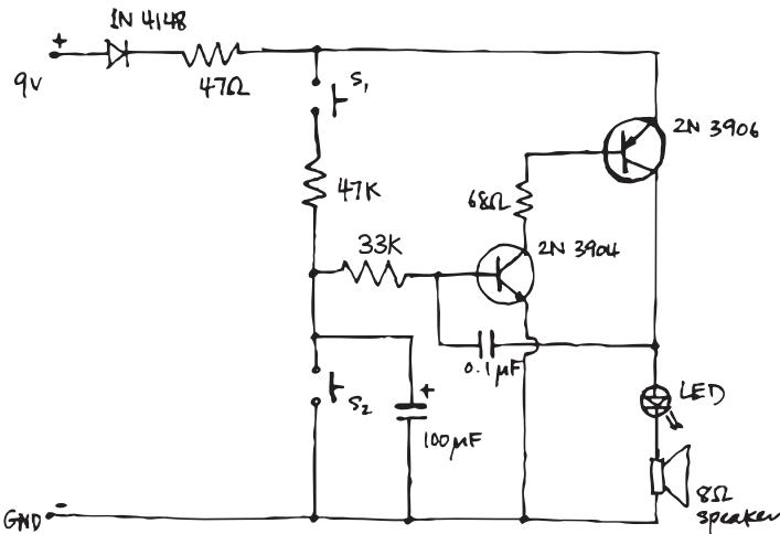
PRESSING SWITCH 2 DISCHARGES THE CAPACITOR DIRECTLY TO GROUND, INSTANTLY STOPPING BOTH SOUND AND LIGHT.
