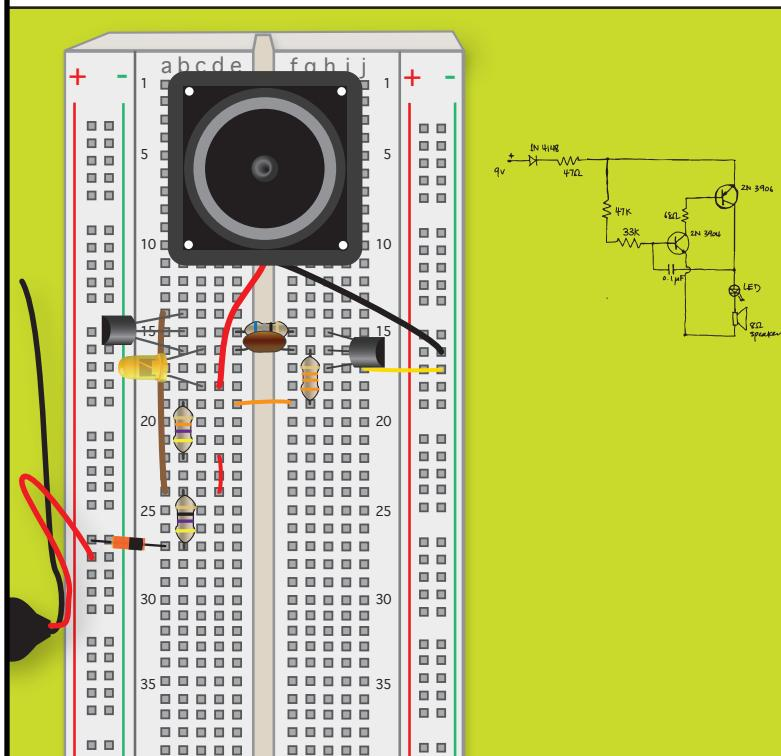
THOUGH IT LOOKS A BIT DIFFERENT, YOU'VE JUST BUILT ANOTHER ASTABLE MULTIVIBRATOR CIRCUIT. REMEMBER THE LED FLASHER CIRCUIT (#2)?
