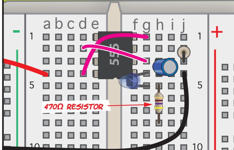
AS ALWAYS, WE NEED A CURRENT-LIMITING RESISTOR IN SERIES TO PROTECT OUR LED FROM DAMAGE. ADD IT NEXT.
