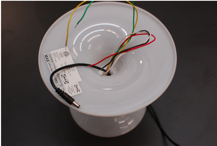
Figure 7-14 Wires going through the base
