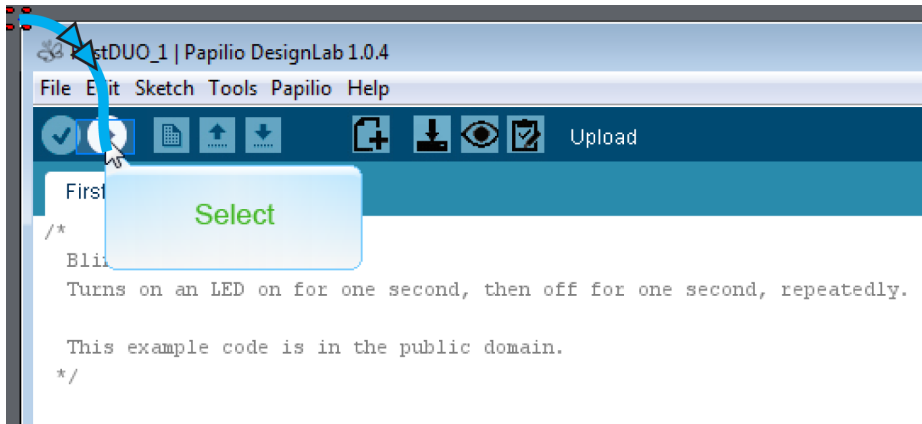
Figure 6-13 Upload your sketch to the ZPUino soft core
