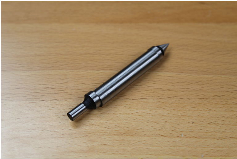
Figure 9-4. Basic edge finder with 1/4-inch shank
