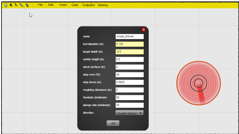
Figure 6-11. Pocket operation to reduce thickness of material
