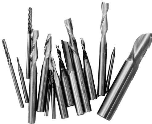
Figure 3-1. An assortment of common end mills
