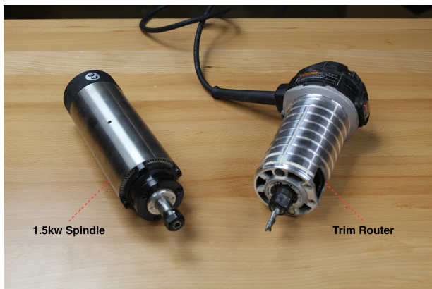
Figure 2-3. 1.5kw air-cooled spindle (left) and trim router (right)
