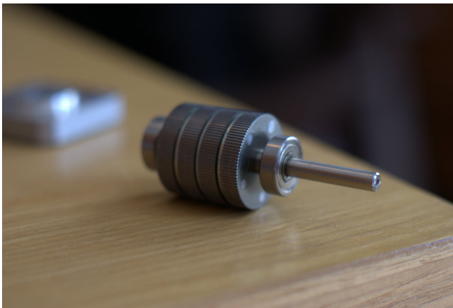
Figure 7-6. Typical stepper motor rotor
