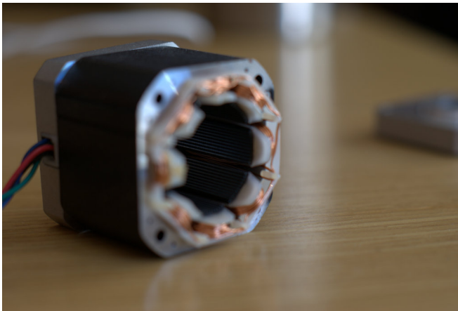
Figure 7-5. Typical stepper motor shell
