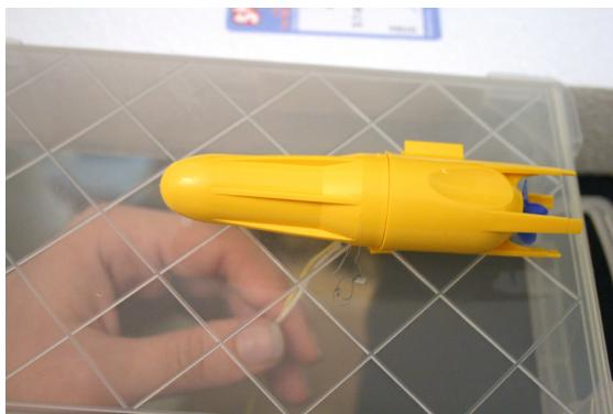
**Figure 3-24** Positioning the motor pod
