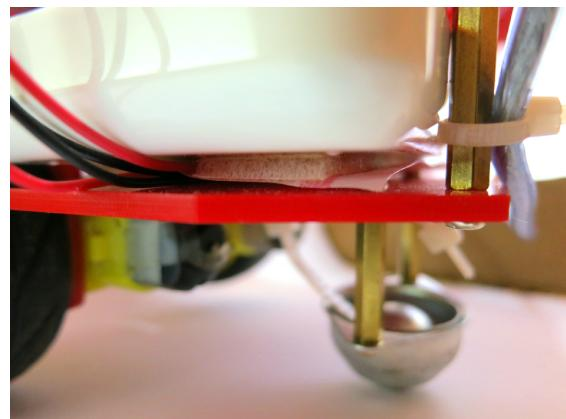
**Figure 4-4** Velcro to hold down the battery
