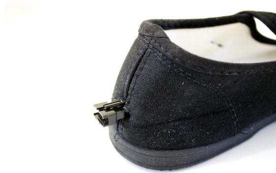
**Figure 14-10** Final assembly of female JST wire within shoe
