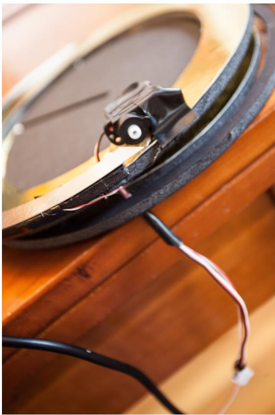
**Figure 7-23** Running the servo and LED wires through the azimuth ring and base disk
