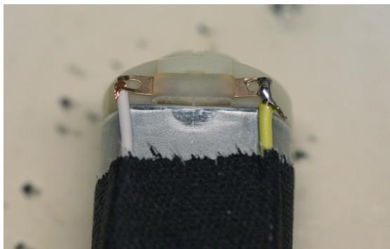
**Figure 3-5** Soldering the wires to the motor
