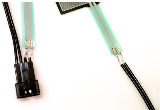
**Figure 14-6** How each pair of wires should look
