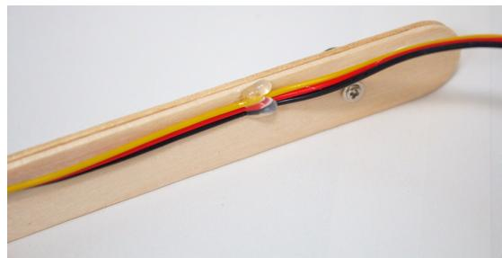
**Figure 2-11** Securing the wrist wire
