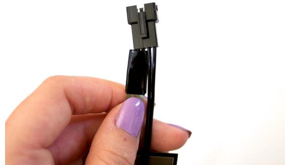
**Figure 14-8** Electrical tape insulates and cushions force applied
