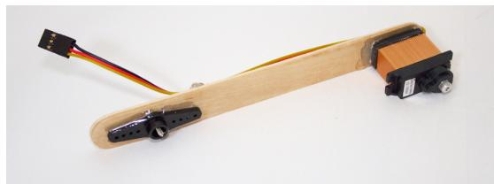
[Figure 2-8](#) Attachment of the wrist servo
