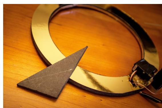
**Figure 7-20** My gnomon, cut for the latitude in Cork, Ireland. The angle on the left is approximately 52° Note my gnomon is not square on the back (right side), and is shorter in the base than 3 inches, so it wouldn't be too tall and interfere with the elevation arc.
