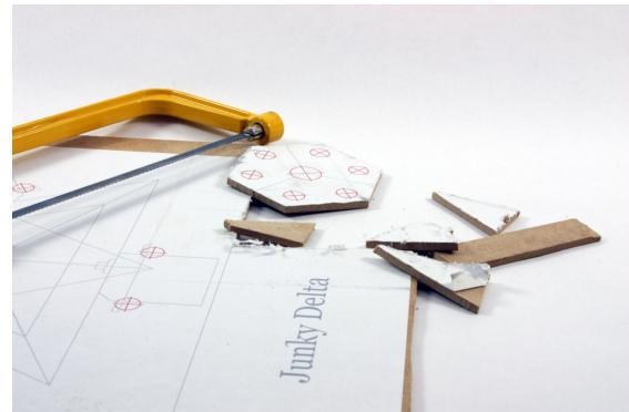
**Figure 13-6** Cutting hardboard
