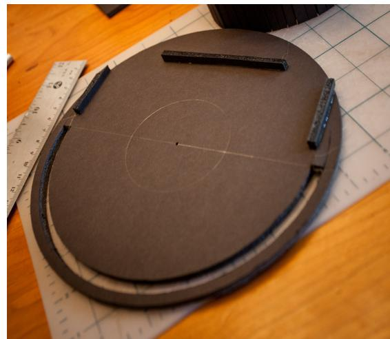
**Figure 7-9** The bottom of the base disk, showing the guides for positioning on the sundial walls
