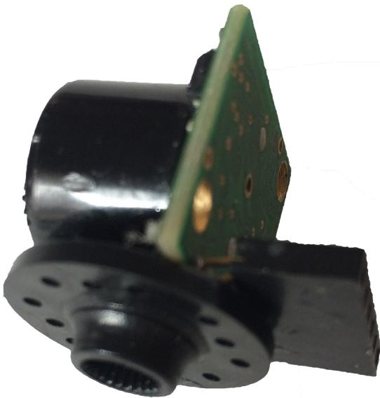
**Figure 12-3** Ultrasonic sensor with servo horn, attached with hot glue
