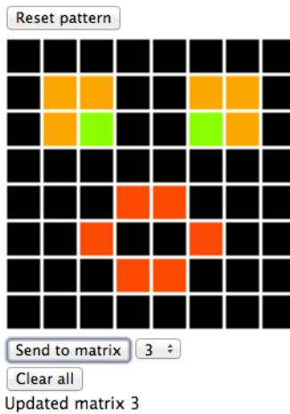
**Figure 8-10** User interface for controlling the matrices
