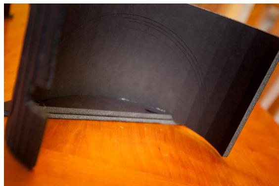
**Figure 7-12** The disk support wall glued to the guide and the foot (note the notch on one side for the Arduino's USB jack)
