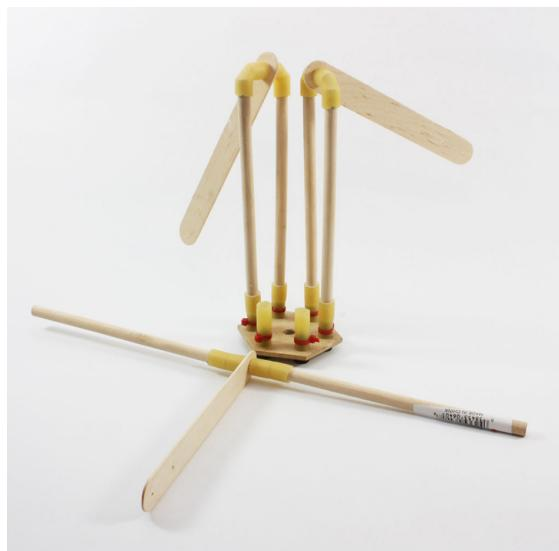
**Figure 13-12** Attaching the end effector
