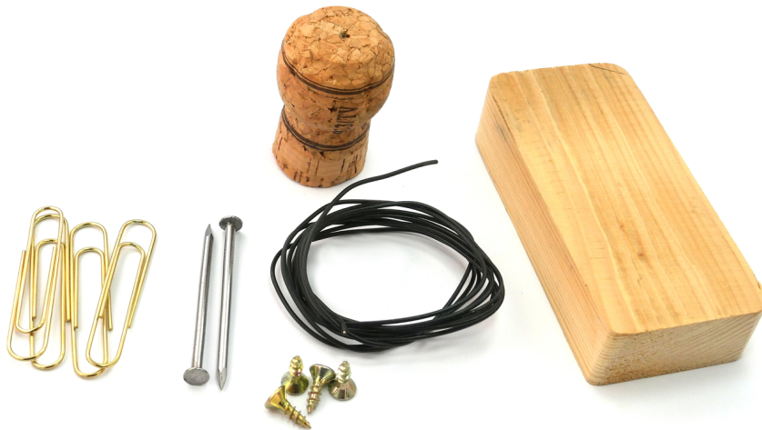
Figure 5-8 The parts you'll need to make a simple motor
