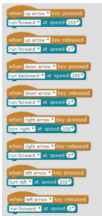
FIGURE 5.1: This Scratch code allows you to control your mBot with the up, down, right, and left keys on your keyboard.
