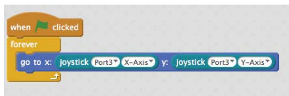
FIGURE 2-20: This single block allows the Me Joystick to move a sprite around the Stage.
