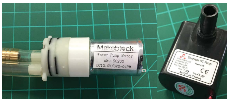
FIGURE 6-4: Makeblock's 12V pump just barely works on mBot motor ports and needs to be kept dry. The black submersible pump is a better choice.
