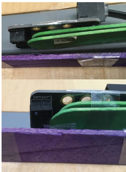
FIGURE 4-27: This popsicle stick solution emerged after students struggled to find a sampling rate that would reliably catch the door in motion.
