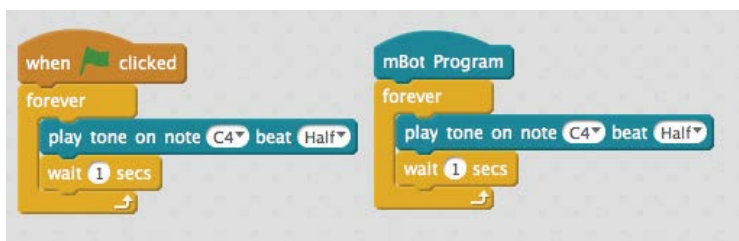
FIGURE 2-29: Only the GreenFlag hat will work when the mBot is tethered, and the mBot Program hat has no effect.
