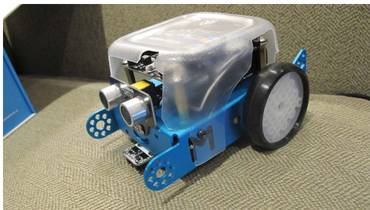
FIGURE 1-10: Case made from 32 oz, 4" × 4" Ziplock container by "John1" on the Makeblock forums
