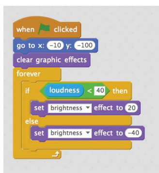
FIGURE 2-14: This block places the green traffic light on the Stage, and then constantly measures the sound level. The light is bright when the sound is low and dark when the volume rises.
