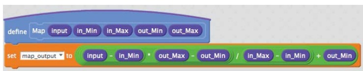
FIGURE 2-24: This custom block re-creates Arduino's map() function. For more information on that function, see https://www.arduino.cc/en/Reference/Map .
