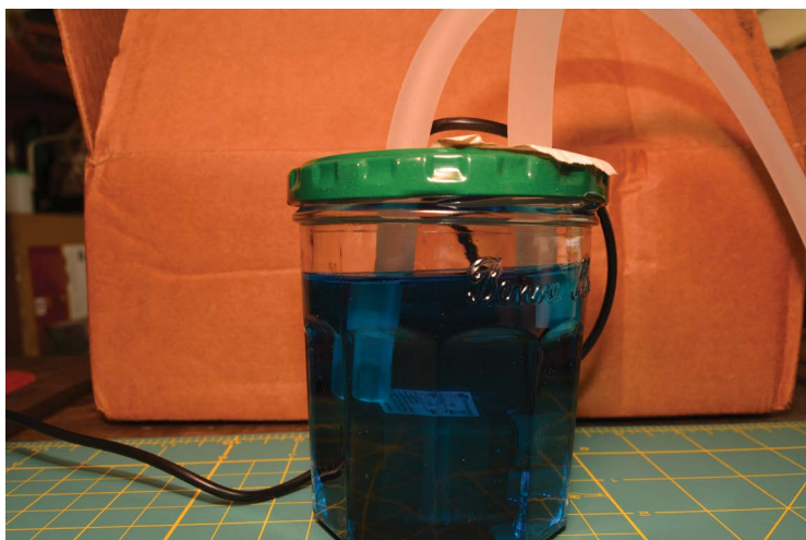
FIGURE 6-8: Here is the completed water reservoir with the tubes attached and the pump on the bottom. You can use food coloring to help you tell from a distance when the water is flowing.
