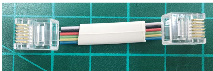
FIGURE 1-11: This is the wrong way to crimp a Makeblock cable!
