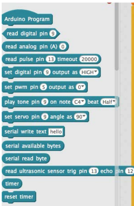
FIGURE 6-28: Programs in mCore can use blocks from the mBot and Arduino extensions simultaneously.
