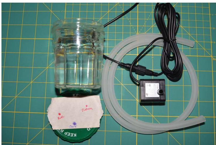
FIGURE 6-5: Here are the parts for the water reservoir. We'll make three holes in the lid: two for the tube and one for the power cable.
