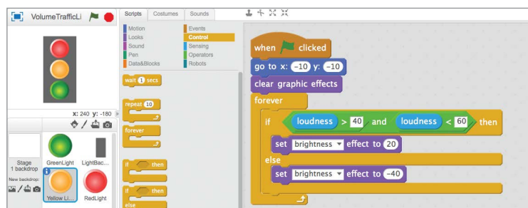
FIGURE 2-17: The green <AND> operator allows us to stack two sensor checks in a single <IF> statement to check for values within a given range.
