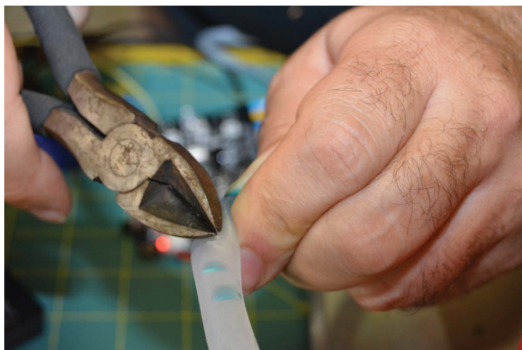
FIGURE 6-15: There's no need to remove lots of plastic. Water pressure will force water out of a small opening.
