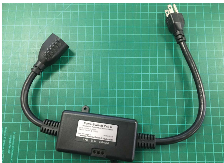
FIGURE 6-33: This PowerSwitch Tail is designed for use with US 110V wall current. There's another version with appropriate plugs for countries using 220V standards.
