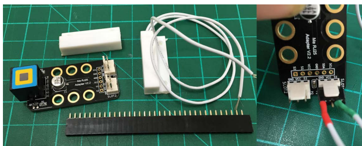
FIGURE 4-29: Soldering header pins to the RJ25 board make almost any crazy switch idea mBot-compatible.
