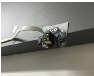
FIGURE 4-26: Early versions of this sensor failed when kindergarten students would only slide the door open far enough to squeak through.
