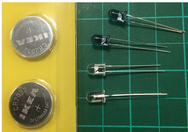
FIGURE 6-10: The top two LEDs use colored plastic to narrow and focus the IR light. Wideband LEDs with clear tops (bottom two) are better for this project but either would work.
