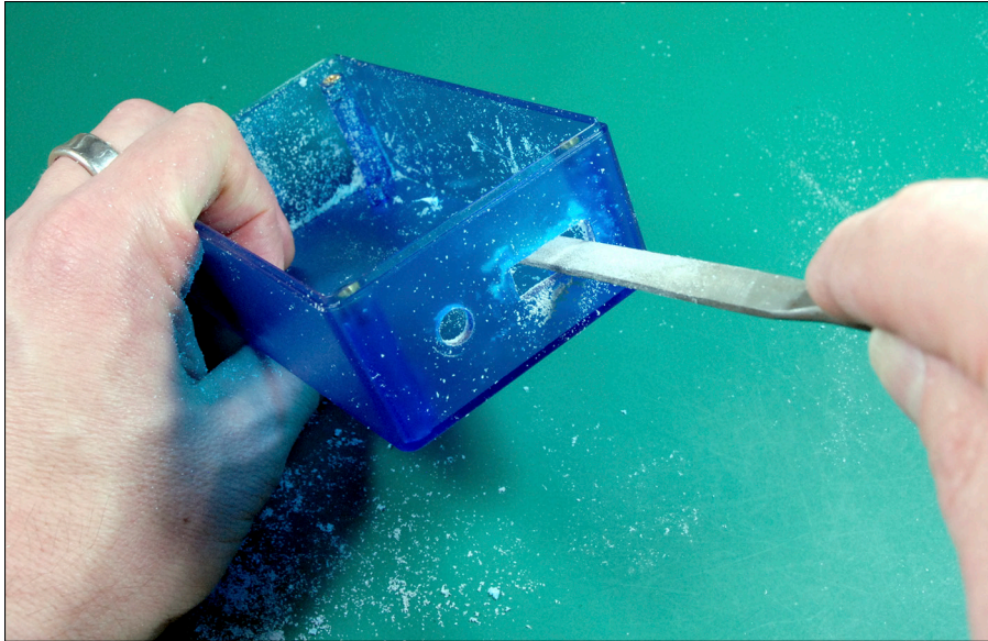
Figure 13-12: Filing the hole for your rocker switch.
