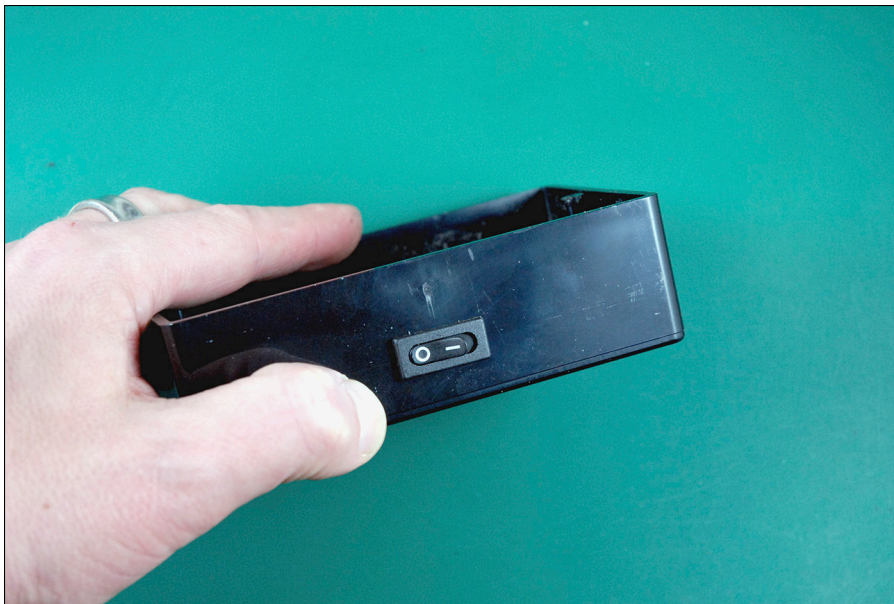
Figure 15-11: Testing the fit of the power switch.
