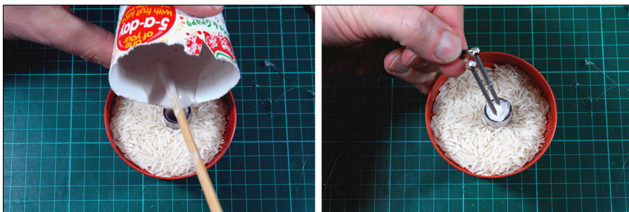
Figure 10-6: Filling the mold with plaster.
