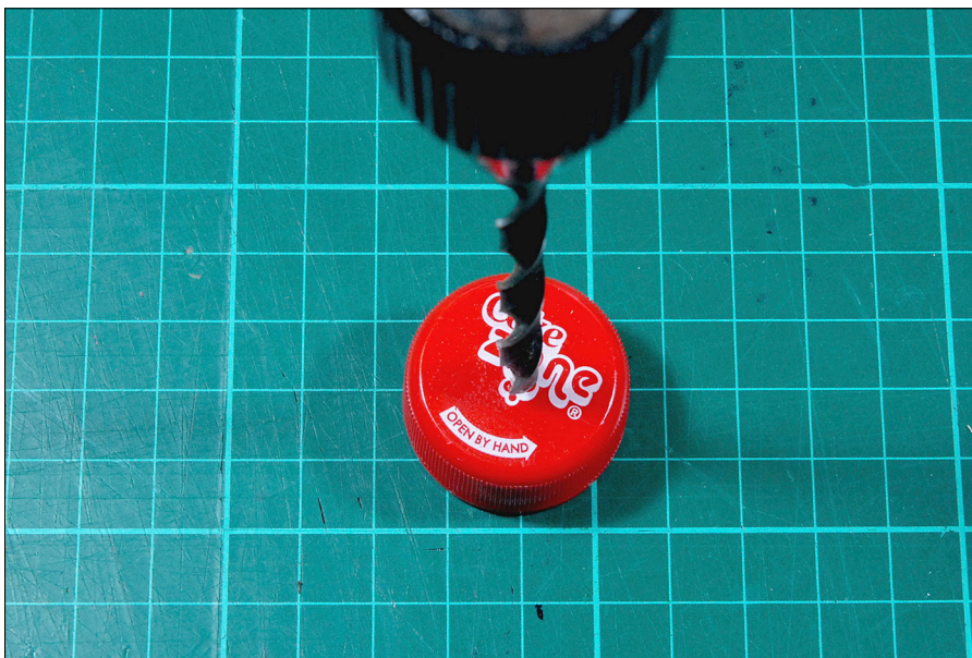
Figure 10-10: Drilling a hole for your supply line.
