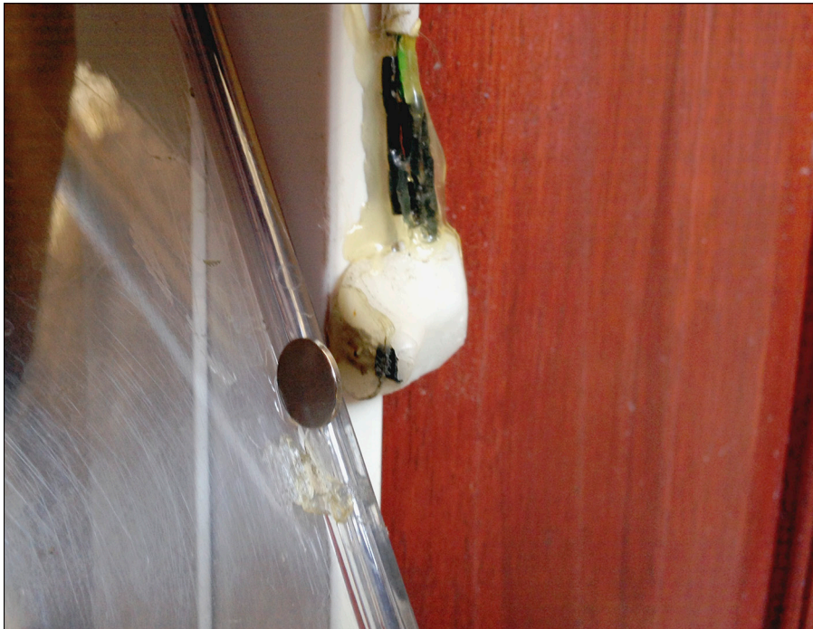
Figure 11-10: Mounting your sen- sors and magnets.
