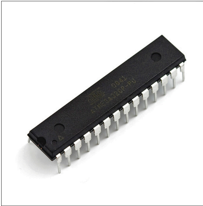
Figure 1-2: The Arduino's brain, an ATmega328 microcon- troller.
