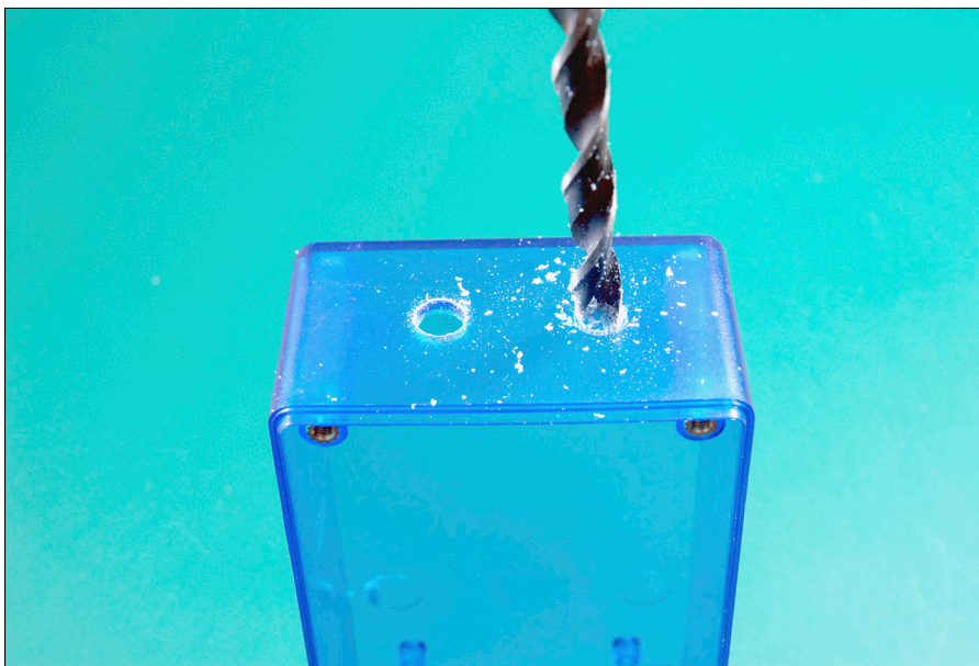
Figure 13-11: Drilling holes for your power switch and antenna.
