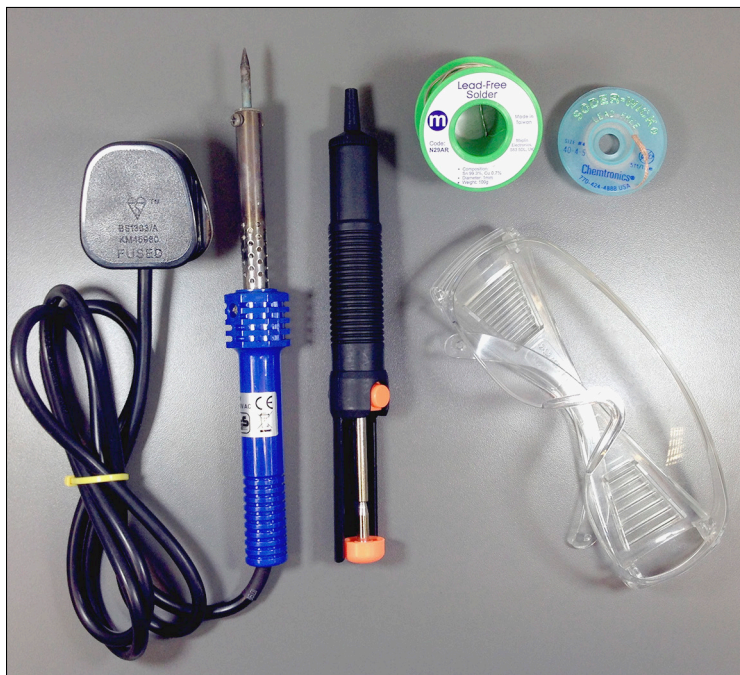
Figure 2-6: An entry-level soldering iron and essential accessories.
