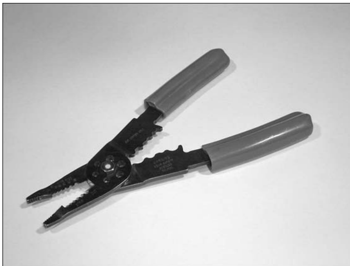
Figure 7-2: This inexpensive hand crimper will make acceptable crimps if used properly.
