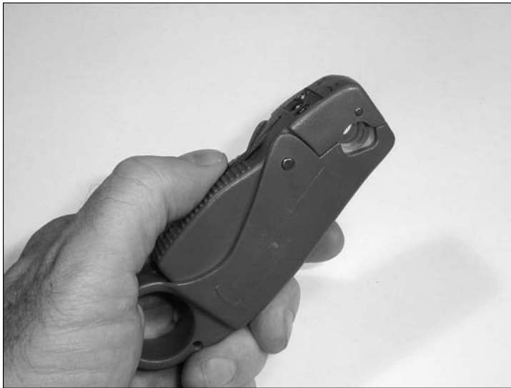
Figure 8-4: A coax stripper “automagically” removes jacket, shield, and center insulation with a few twists — a big time-saver!
