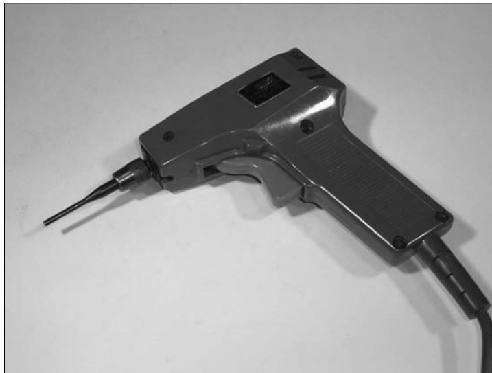
Figure 6-6: A motorized wrapping tool saves a great deal of effort when constructing complex circuits or if you will do a lot of wire-wrapping.
