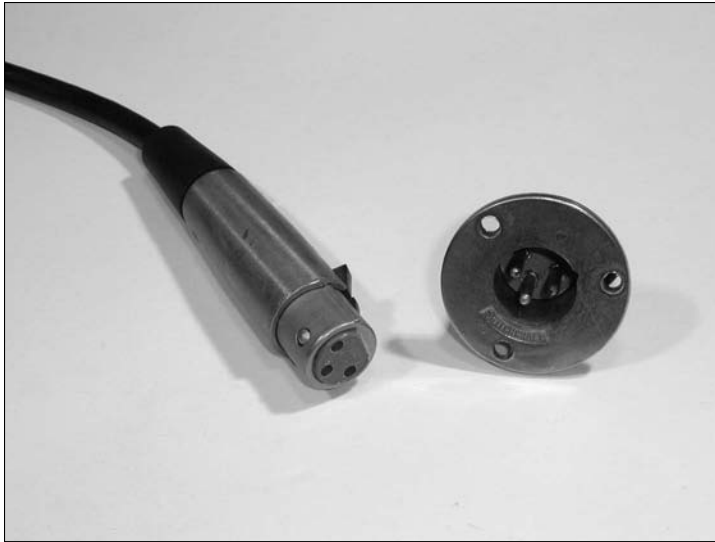
Figure 10-1: XLR connectors are the standard for professional and public-address system microphone and audio wiring.
