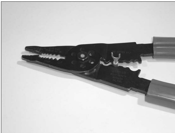
Figure 7-5: Place the crimping in the middle of the terminal's barrel on the opposite side of the barrel's seam.
