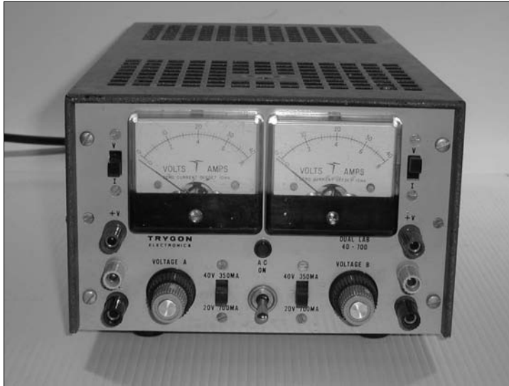
Figure 11-3: A dual lab supply has two internal power supplies, completely isolated from each other and usable independently or combined.
