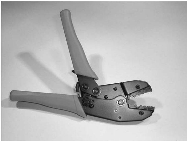
Figure 8-2: The coaxial connector crimping tool compresses the pieces of the coax connector to make a consistent that maintains its integrity at radio frequencies.
