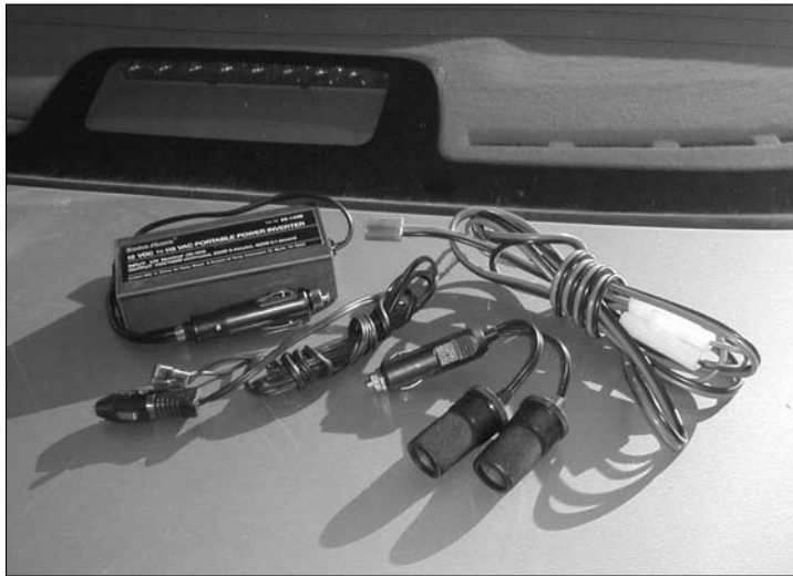
Figure 16-1: Vehicle power sources include lighter plugs and DC to AC inverters.
