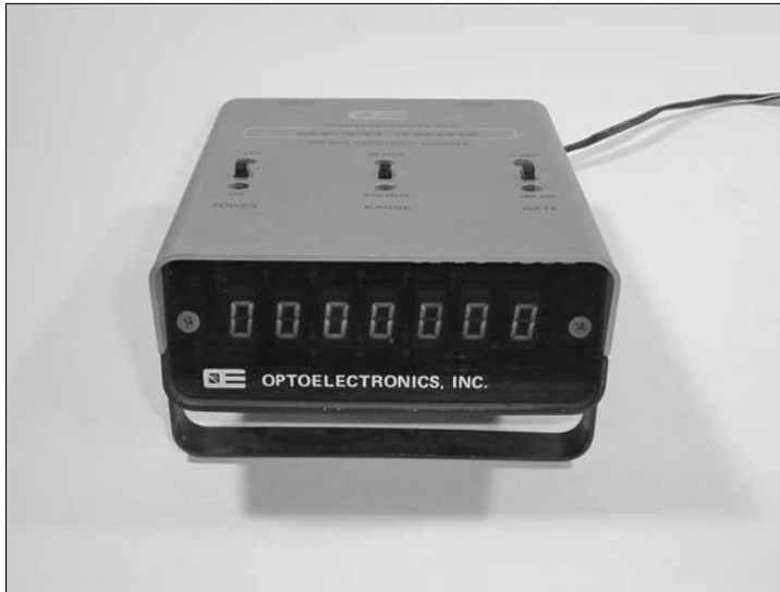
Figure 11-6: A basic counter used for field and bench measurements. Designed for use with radio signals, this counter shows frequencies as high as 500 MHz.
