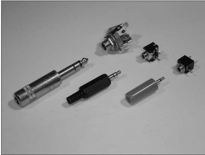
Figure 10-3: Phone plugs come in three sizes: 1/4", miniature 1/8" (or 3.5 mm), and subminiature 2 mm. They are used for audio and control connections. Their mating jacks are shown to the right of each plug.
