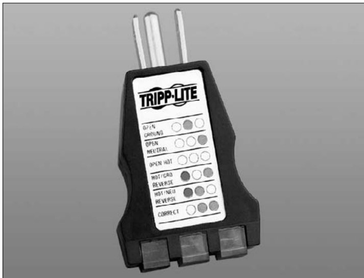
Figure 13-3: An AC socket tester quickly identifies a number of faults, including a “dead” socket.
