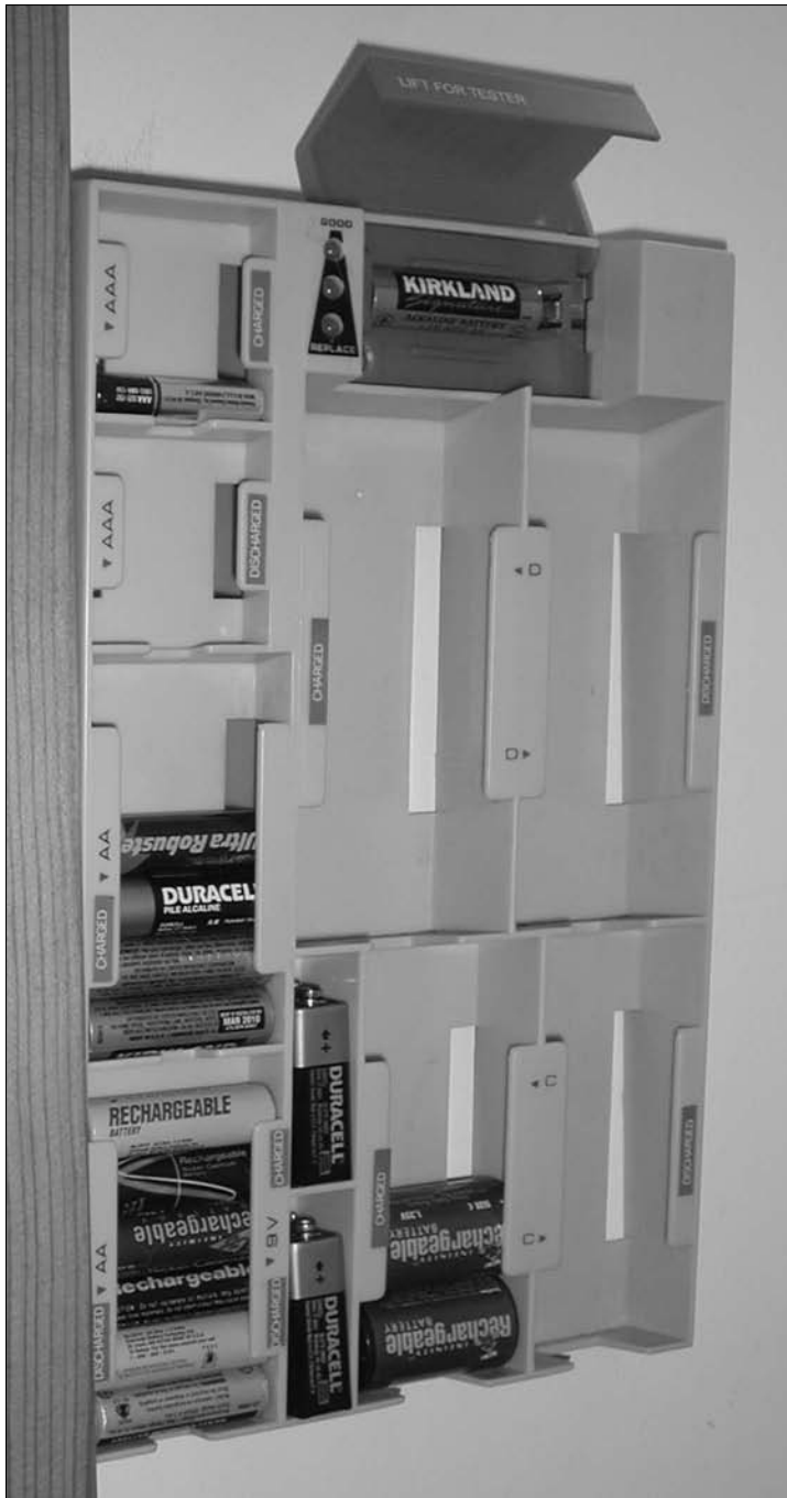
Figure 13-4: A battery tester applies a small load to the battery when measuring battery voltage, causing the voltage from weak batteries to drop, which identifies a marginal battery that would otherwise test as good.
