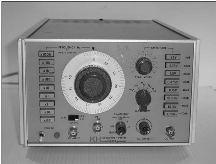
Figure 11-5: Function generators produce waveforms used in testing and developing circuits. The frequency and amplitude of the output are continuously adjustable over a wide range.
