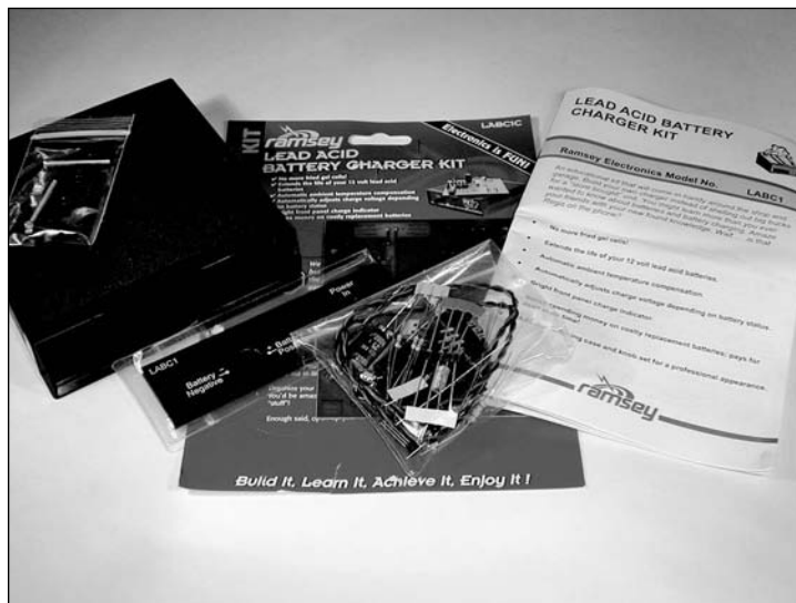
Figure 4-1: The battery charger kit uses a typical through-hole board. The components have either wire leads or terminals that stick through the board and are soldered to exposed pads on the bottom of the board.
