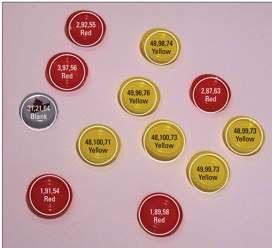
Figure 11-4: Circle and color detection with OpenCV.
