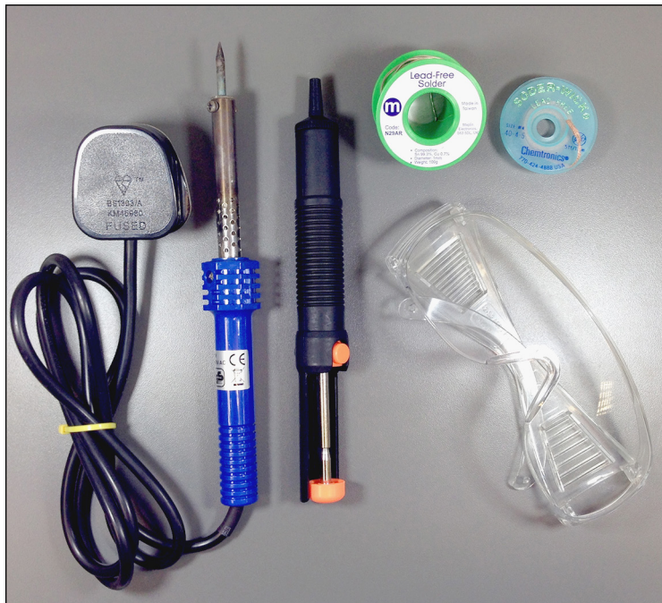
Figure 2-3: An entry-level soldering iron and essential accessories.
