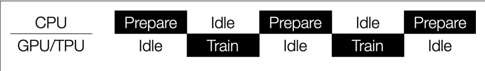
Figure 6-1. GPU starvation, while waiting for CPU to finish preparing the data
