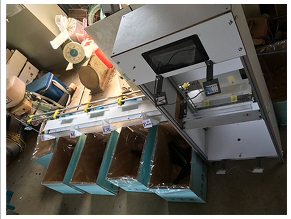
Figure 15-14. Makoto Koike's cucumber sorting machine ( image source )
