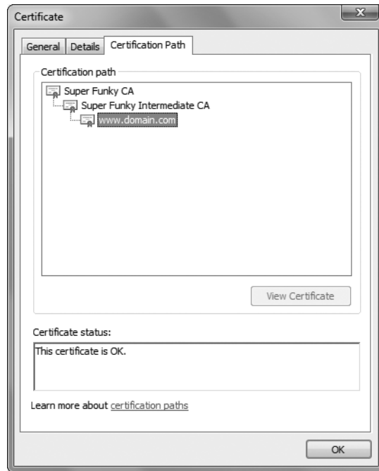
Figure 7-21: The chain of trust for www.domain.com
