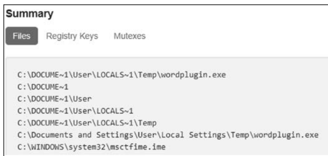
Figure 3-5: The Files tab of the Summary pane, showing which files our malware sample modified
