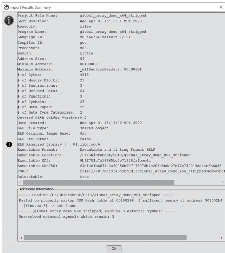
Figure 13-4: Import Results Summary window for an ELF binary
