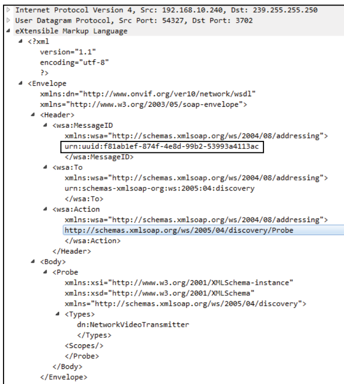
Figure 6-16: The WS-Discovery Probe from exacqVision, output by Wireshark
