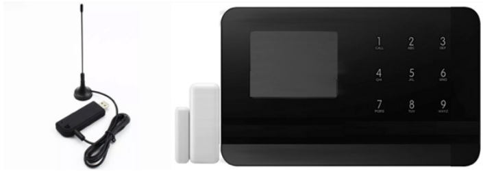
Figure 15-1: A cheap RTL-SDR DVB-T dongle and an alarm system with a wireless door access sensor
