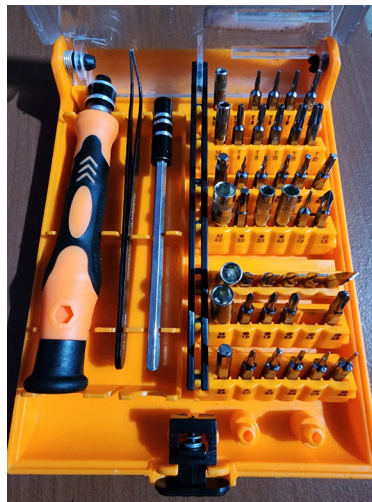
Figure 7.1 – Toolkit with various tips for opening devices and drives
