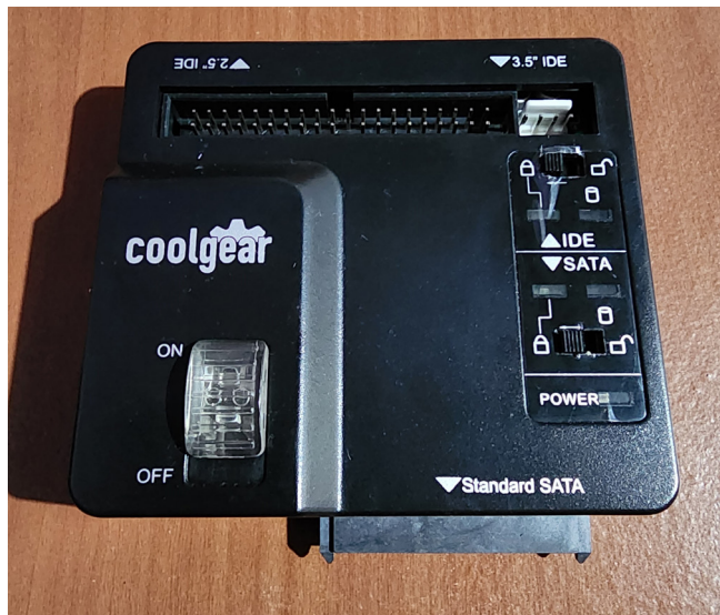
Figure 7.6 – USB to SATA and IDE write-blocker device
