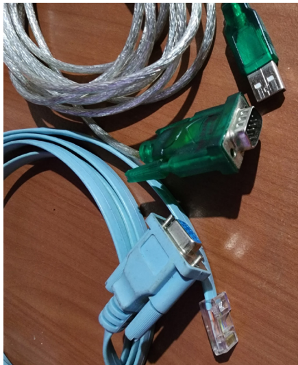
Figure 7.4 – Serial to RJ-45 (left) and Serial to USB (right) cables
