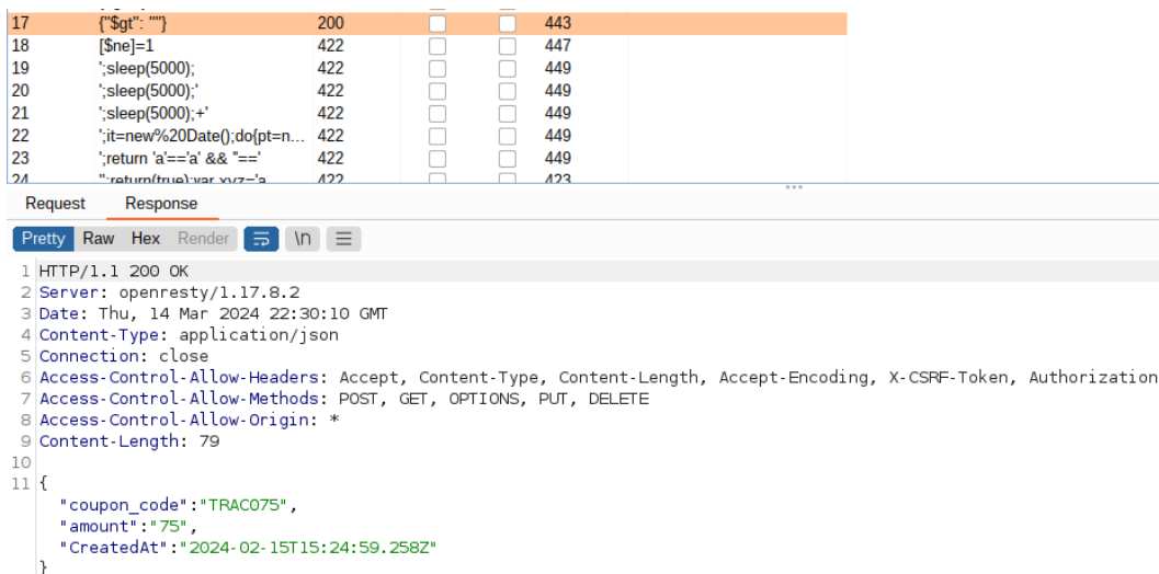
Figure 5.8 – crAPI disclosing a coupon code after a NoSQL injection attack
