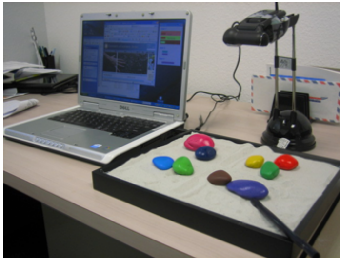
Figure 5.1: Prototype of the Japanese Garden, a tangible interface to manage interruptions.
