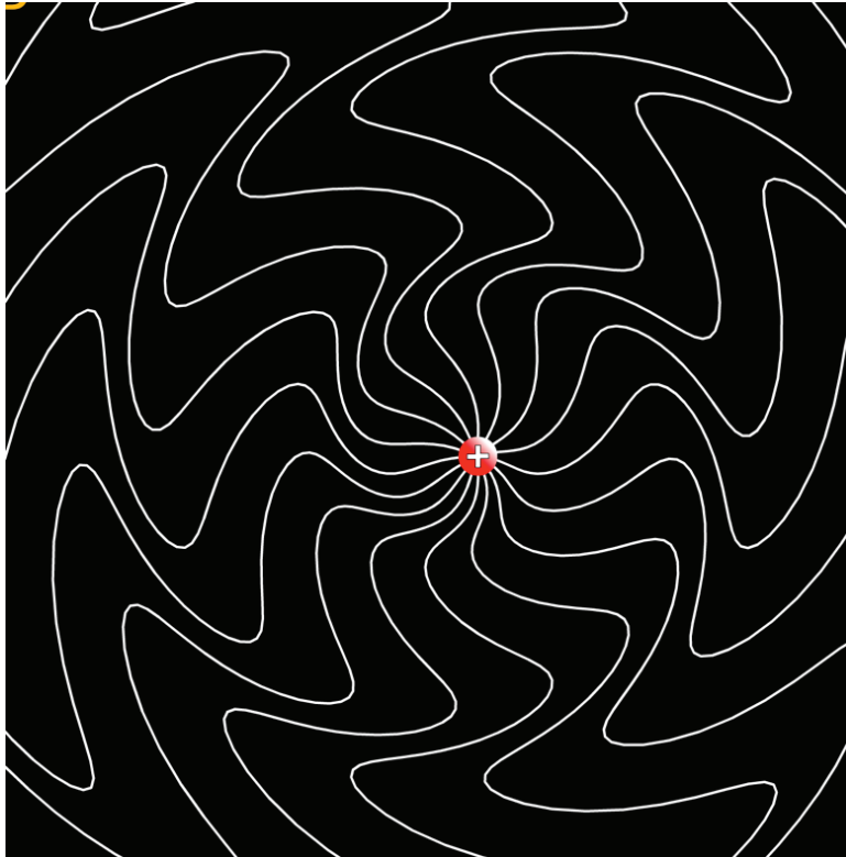
Figure 2.1: Electric field produced by an accelerating charge.
