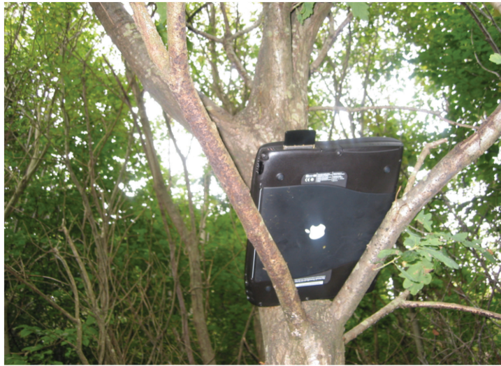
Figure 4.4: A laptop placed between branches of a tree to provide an aerial as part of the makeshift infrastructure.
