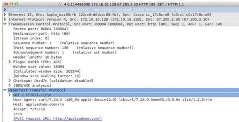
FIGURE 13.1 A Simple HTTP GET Request Packet Shown in Wireshark
