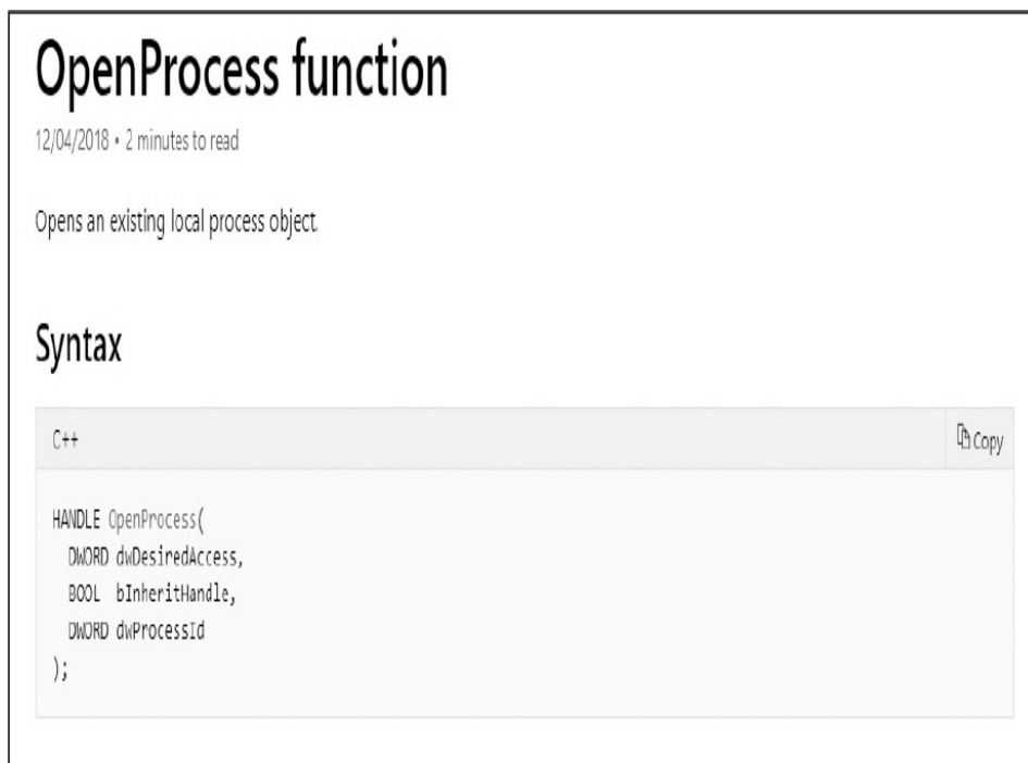
Figure 12-1: The Windows API object structure for OpenProcess()
