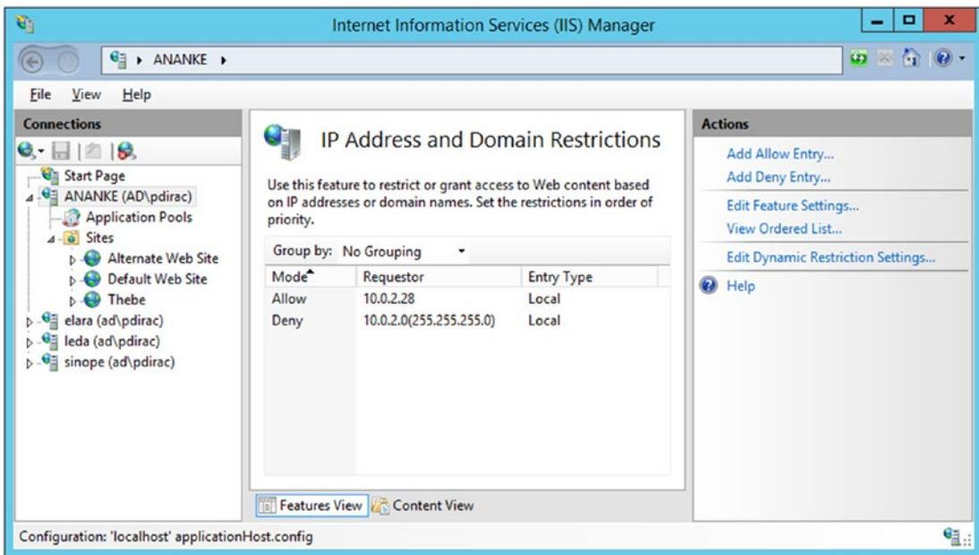
**Figure 15-5.** IP Address and Domain Restrictions on Windows Server 2012 R2
