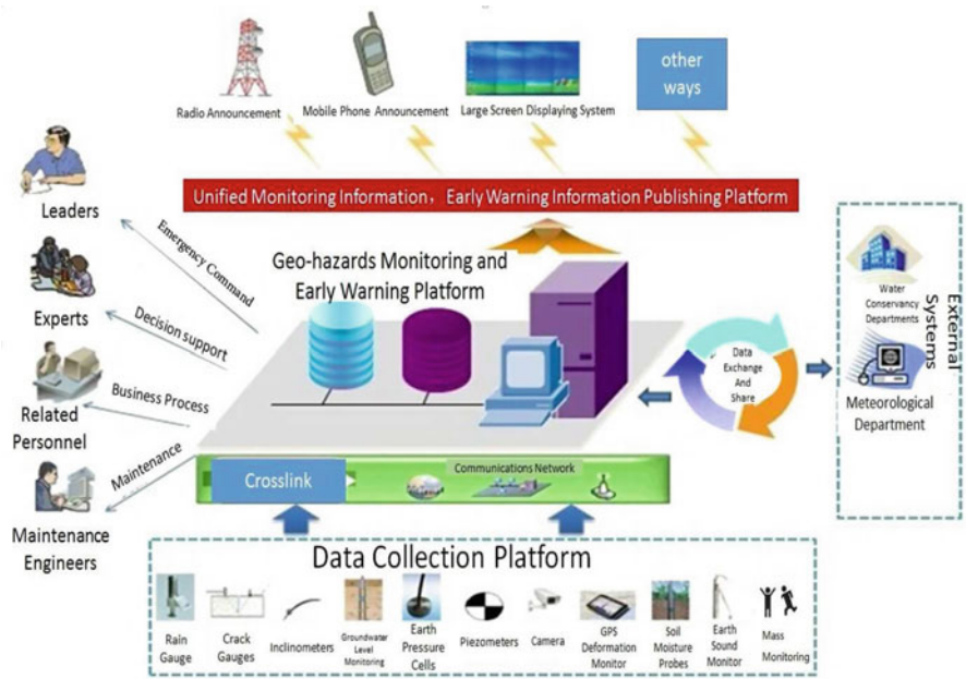
Fig. 3.10 Diagram of the monitoring and early warning platform
