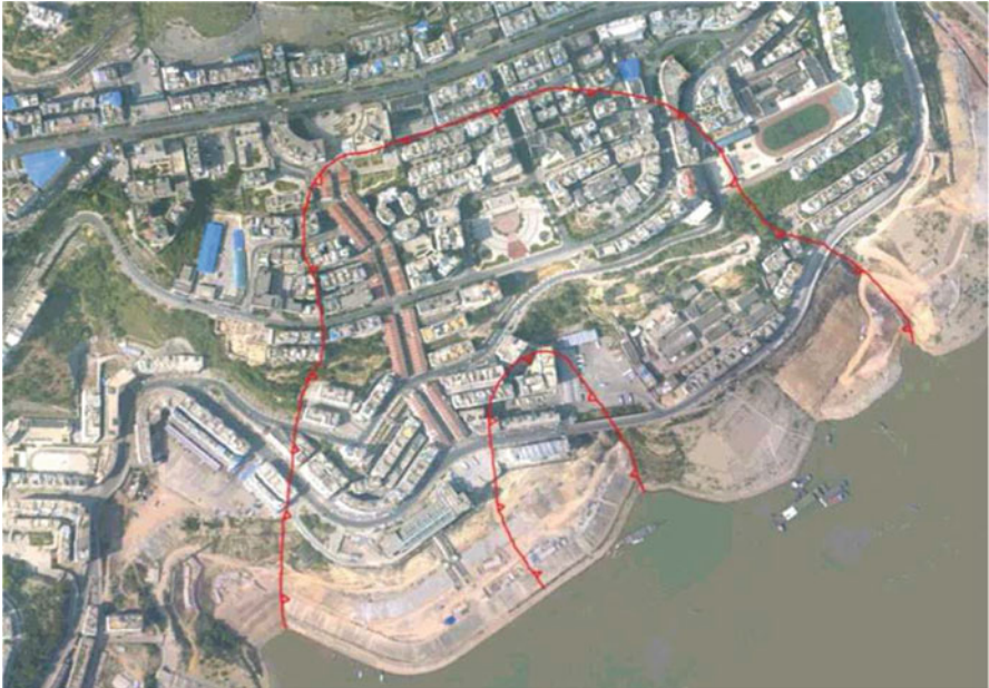
Fig. 3.2 Identify a landslide from remote sensing images
