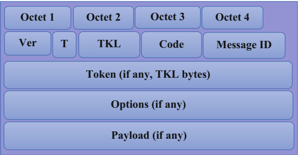
Fig. 7.6 Constrained Application Protocol (CoAP) message format
