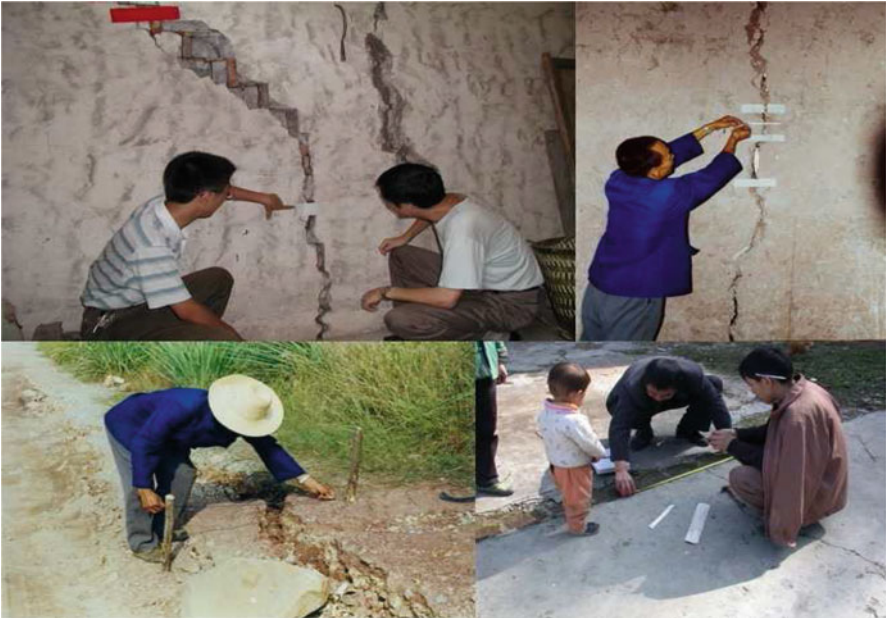
Fig. 3.9 Scraps of paper to monitor wall crack (the upper figures) and a tape to measure the length of landslide rapture (the lower figures)
