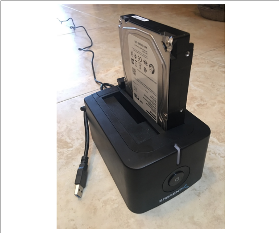
Figure 2-3. An example of a SATA-to-USB adapter, showing the cartridge-like approach to connecting an internal drive to a computer via external USB.
