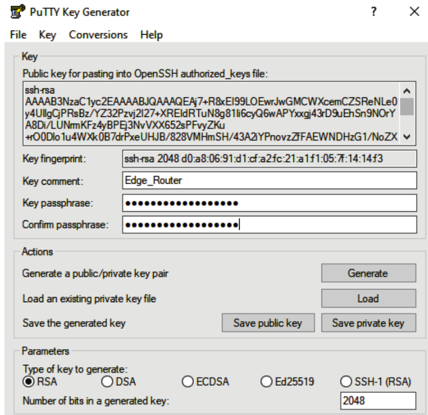
Figure 9.4 – Using PuTTYgen to generate a public/private key pair
