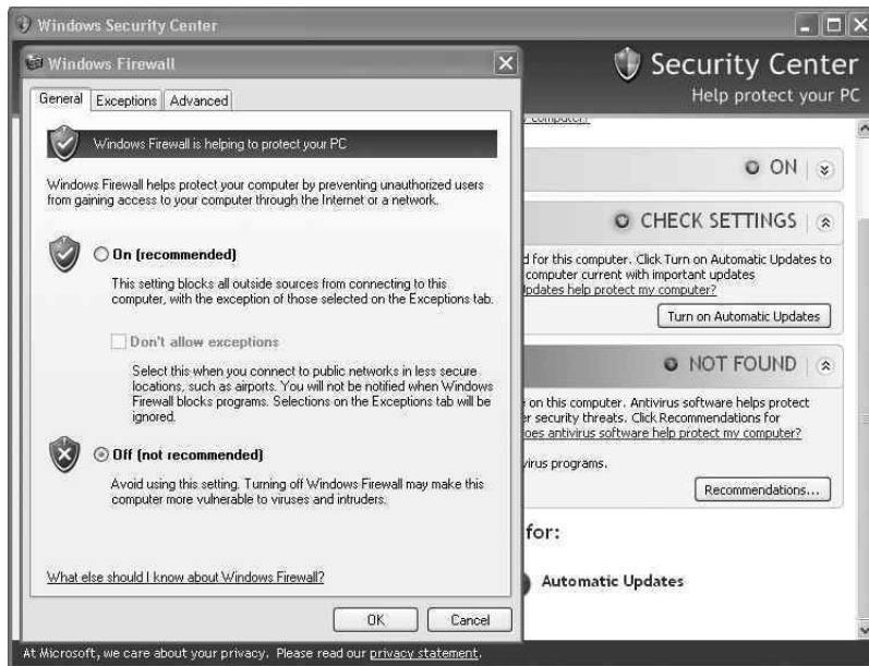
Figure 1-33: Turning off the Windows firewall
