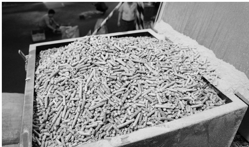
Compressed sawdust pellets, used to fuel the ingot smelter
