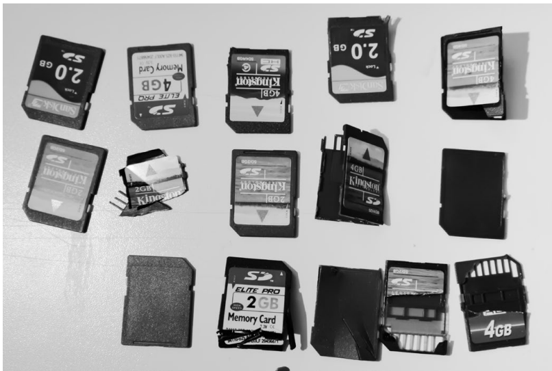
Some of the eggs—or rather, SD cards—we cracked open to find the vulnerability
