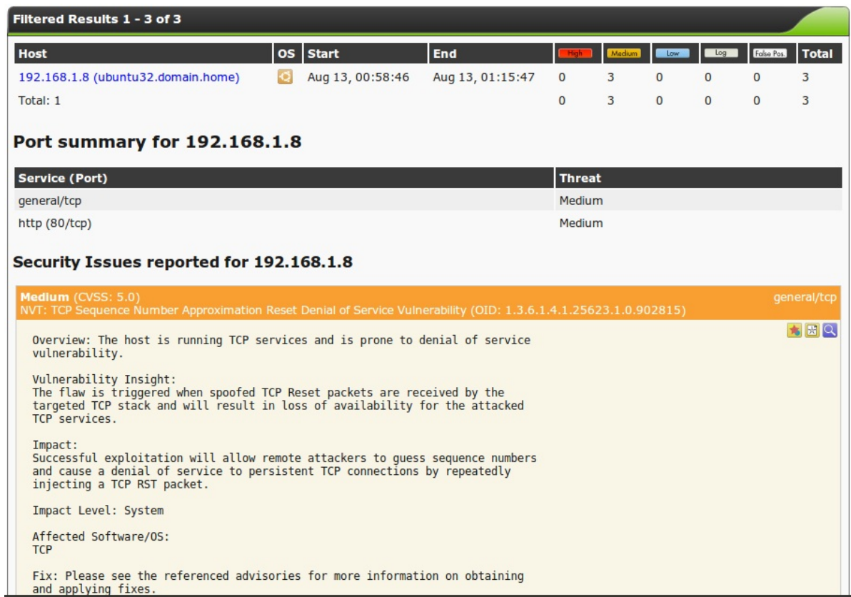
Figure 5-5. Greenbone web interface for OpenVAS showing three “medium” vulnerabilities for a scan target
